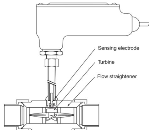
Figure 2.2 Inline Turbine flow meter, (Montgomery & McDowall 2009)
