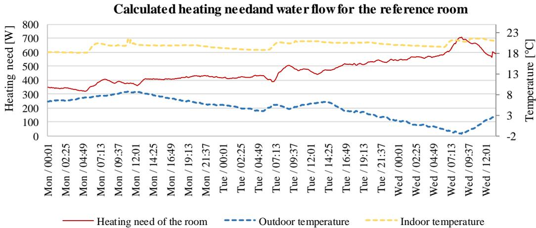
Graph 3.18 Calculated heating need for the test room over the period of three days
