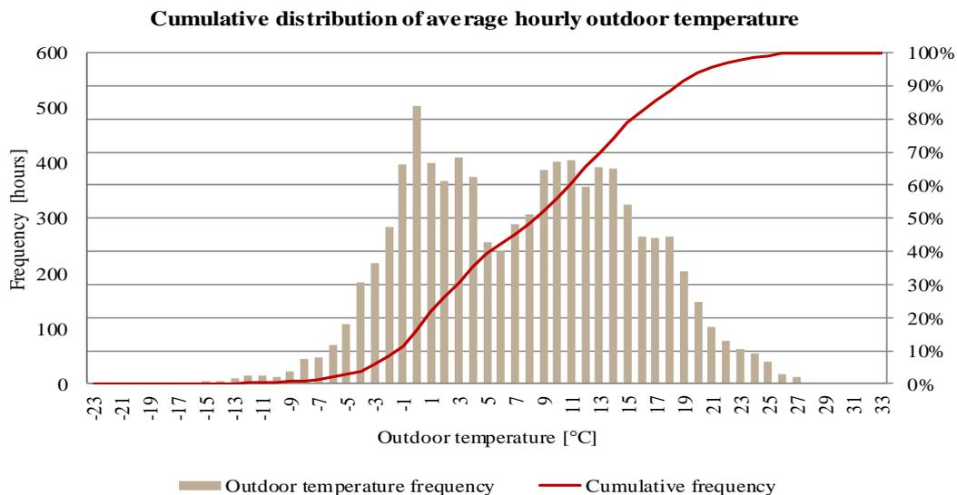
Graph 2.12 Cumulative curve for outdoor temperature in Denmark, from DRY 2013 in BSim
