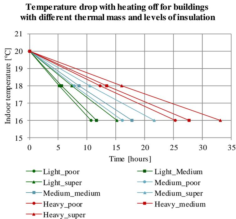
Graph 2.7 Time to reach setback temperature for buildings with different thermal mass and levels of insulation
