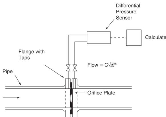
Figure 2.1 Orifice Plate flow meter, (Montgomery & McDowall 2009)
