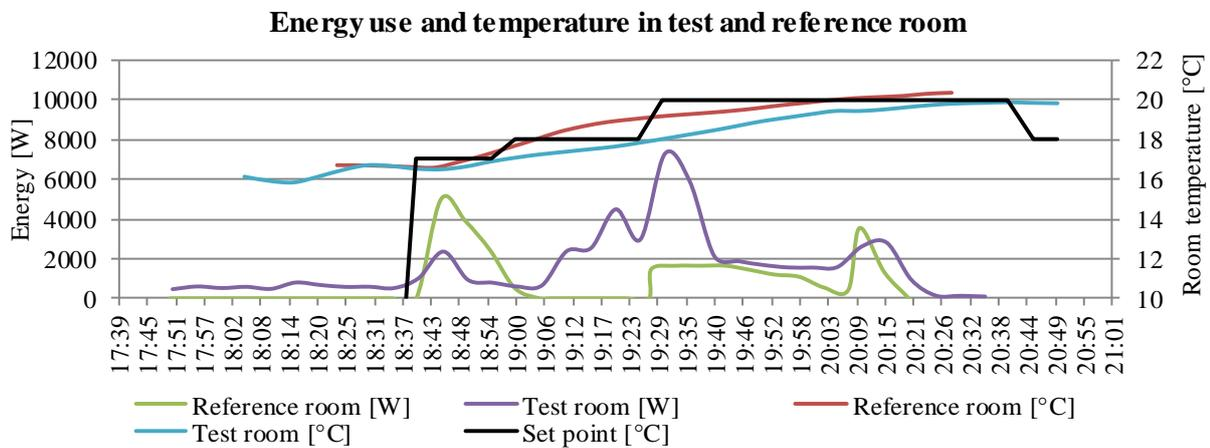
Graph 3.9 Resulting energy use of both meters, and operative temperature in test and reference room
