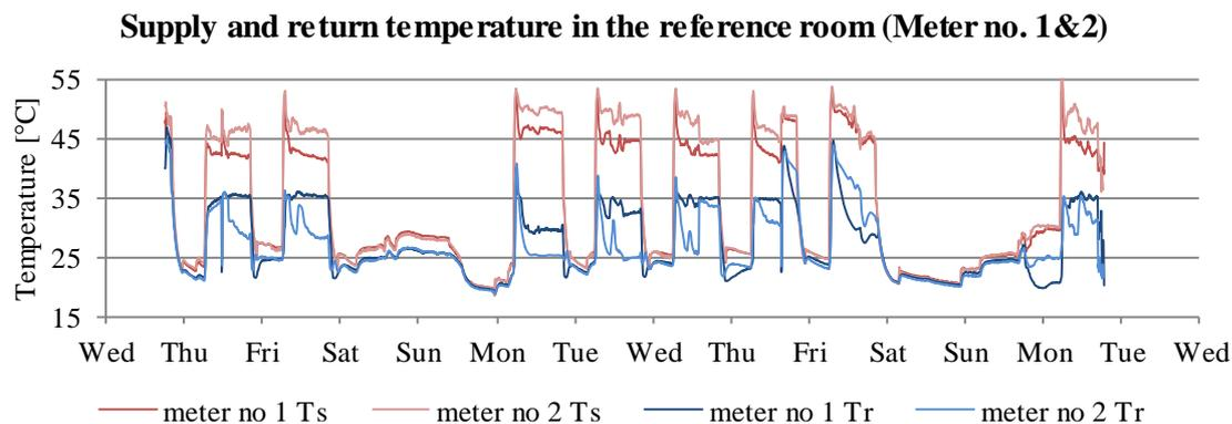
Graph 3.16 Supply and return temperature measurements over two weeks in the reference room
