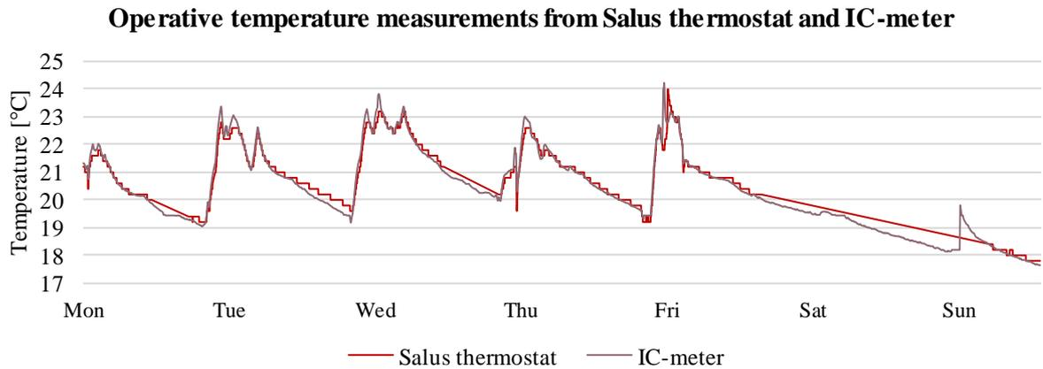
Secondly, the information logged by Salus Controls is analysed graphically with the aim of understanding the operation of the TRVs. The graph below shows operative temperature, thermostat set point and the percentage of valve opening in the test room for the period of one week. It should be noted that there are two TRVs installed in the room, and their opening percentages are exactly the same, since they both are controlled by one room thermostat.
