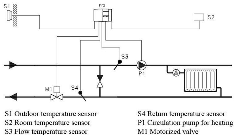
Figure 3.11 Heating system- connection to ECL (Danfoss n.d.)
