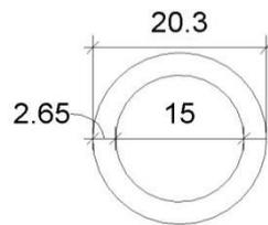
Figure 3.20 Pipe dimensions for the test
