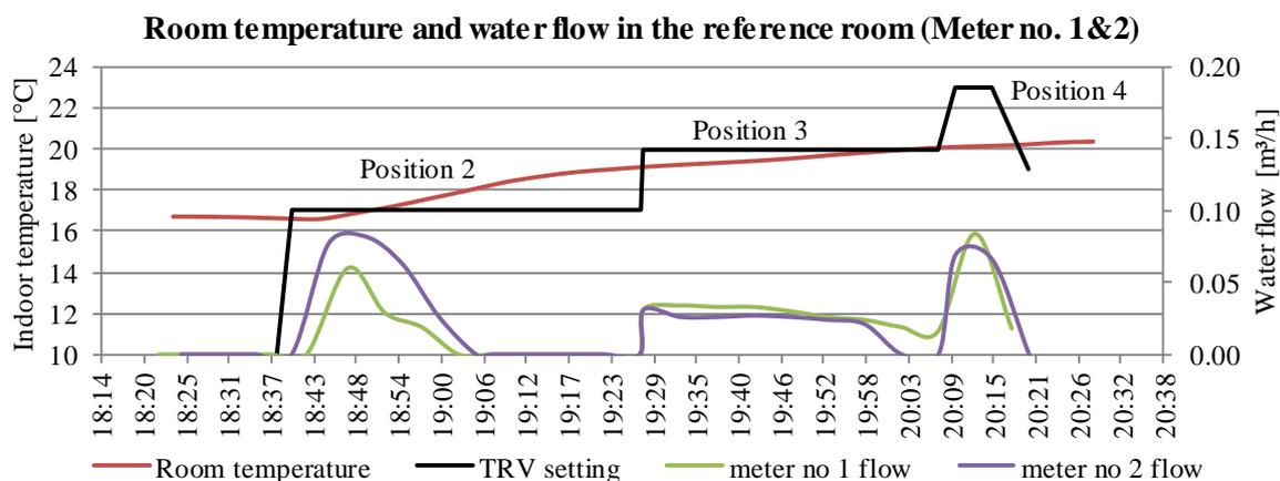
Graph 3.6 Testing the setpoints of the existing TRVs in the reference room
