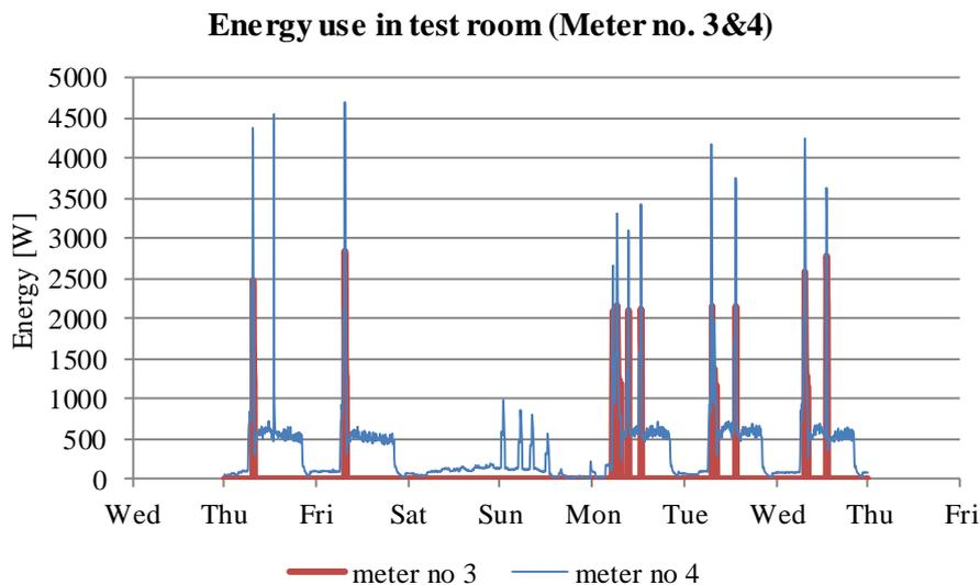
Graph 3.11 Energy use of the two radiators in the test room over a period of one week
