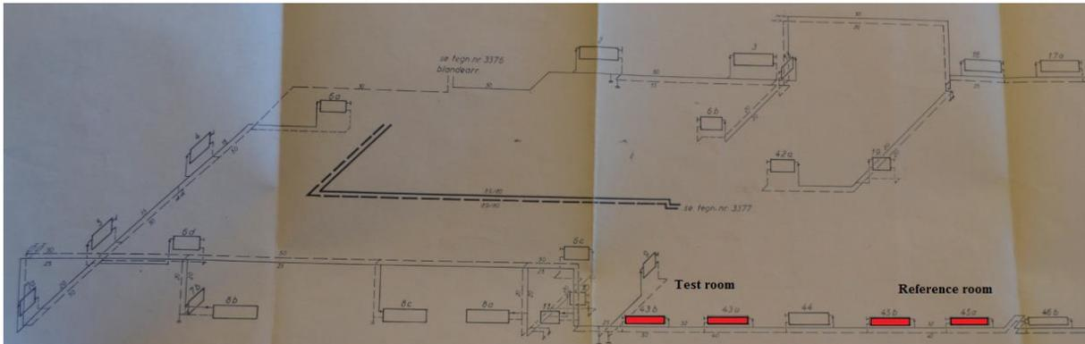
Figure 3.5 Distribution pipes: reverse return heating system
