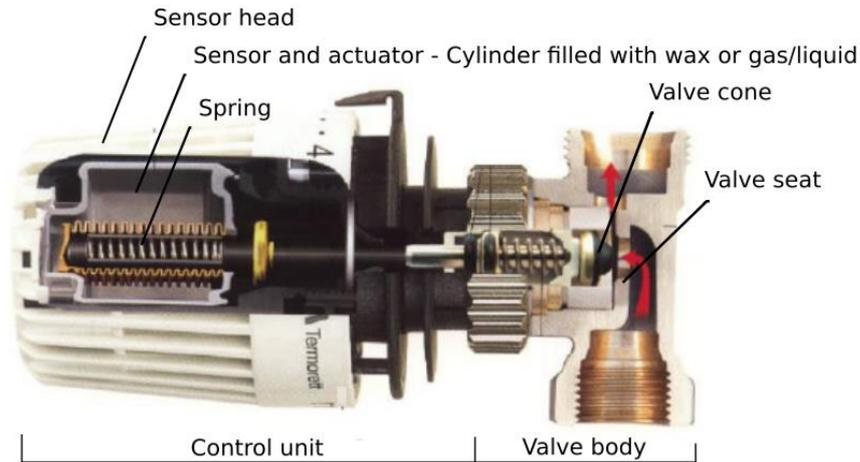
Figure 2.7 Section of a thermostatic radiator valve, photo taken from (Pomianowski 2015)
