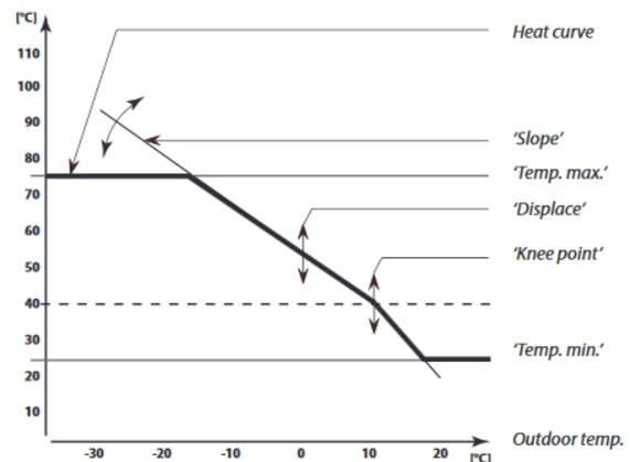
Graph 2.2 Parameters of a heat curve (Danfoss 2008)
