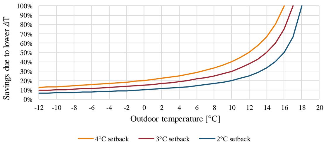
Graph 2.3 Effect of applying different setback temperatures to the heat loss
