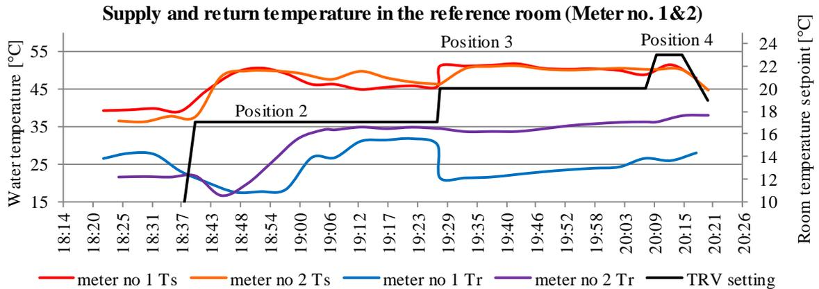
Graph 3.7 Testing TRV positions in the reference room: resulting supply and return temperatures
