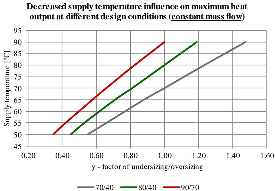
Graph 2.16 Decreased supply temperature influence on heat output at different design conditions (mass flow kept constant)
