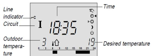
Figure 3.13 Display C example from (Danfoss n.d.)
