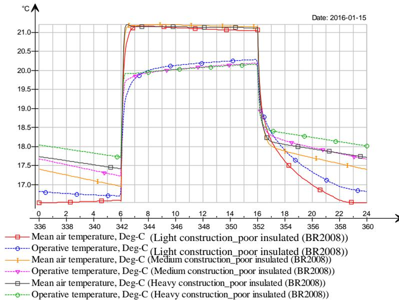
Graph 2.10 Indoor temperatures for light, medium, heavy buildings with insulation level (BR2008)
