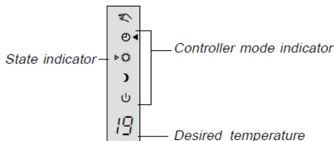
Figure 3.14 Controller modes (Danfoss n.d.)
