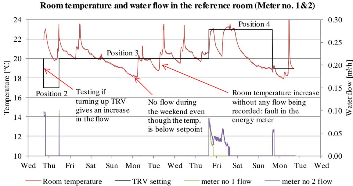
Graph 3.15 Testing different positions on TRVs in the reference room over a longer period of time
