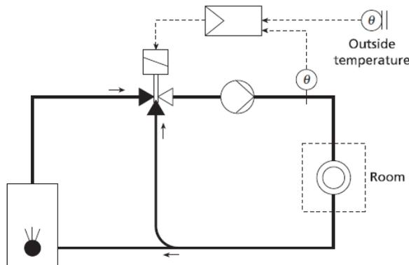
Figure 2.13 Weather compensation for controlling flow temperature (CIBSE 2010)
