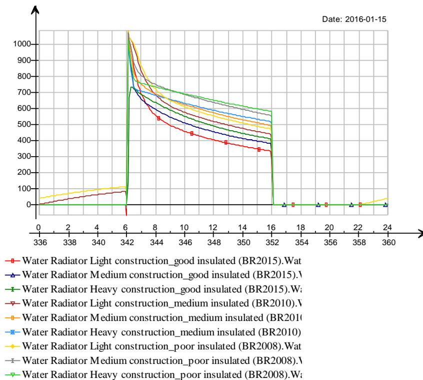
Graph 2.11 Radiator output in watts for one day (at outdoor -12°C)
