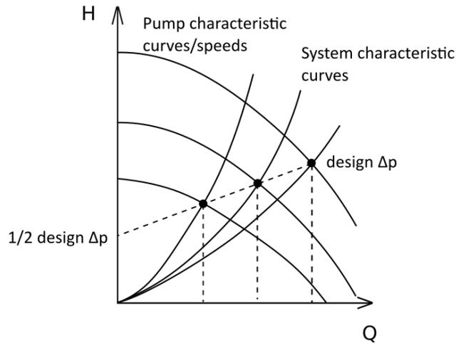
Figure 2.12 Pump with a proportional pressure regulation: pressure decreases with decreasing flow
