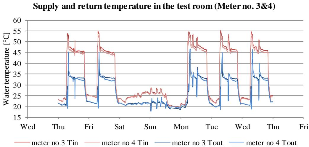
Graph 3.12 Supply and return temperatures in the test room over a period of one week
