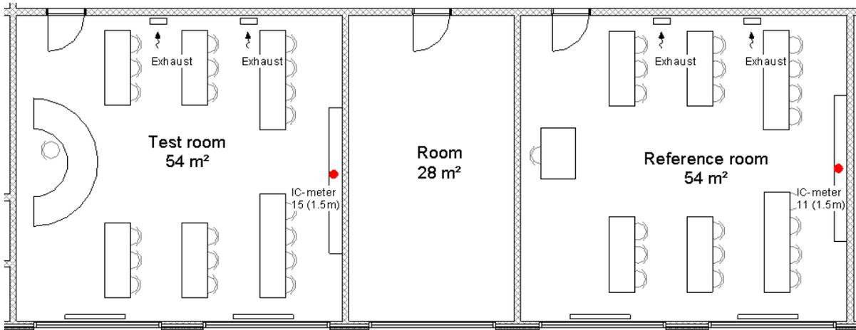
Figure 3.16 Placement of Indoor Comfort sensors
