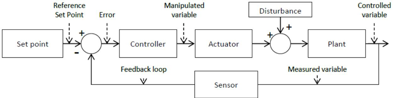
Figure 2.14 Block diagram of closed loop control
