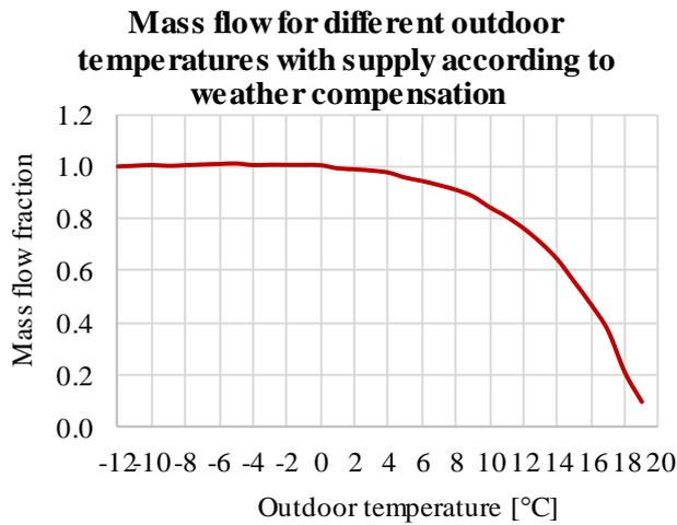
Graph 2.21 Mass flow fraction depending on outdoor temperature; applied supply temperature reduction according to weather compensation
