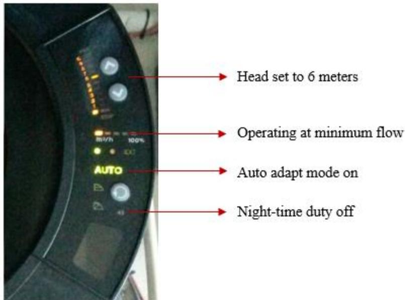
Figure 3.10 Picture of the control panel of the pump
