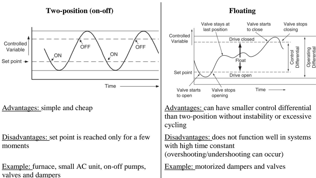
Table 2.2 Examples of different control types (a). Illustrations' source: (Montgomery & McDowall 2009)
