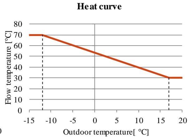
Graph 2.22 Simple heat curve. Supply temperature decreases proportionally to the outdoor temperature increase
