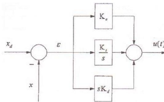
Figure 2.15 Block diagram of a classic PID controller (Manring 2005)
