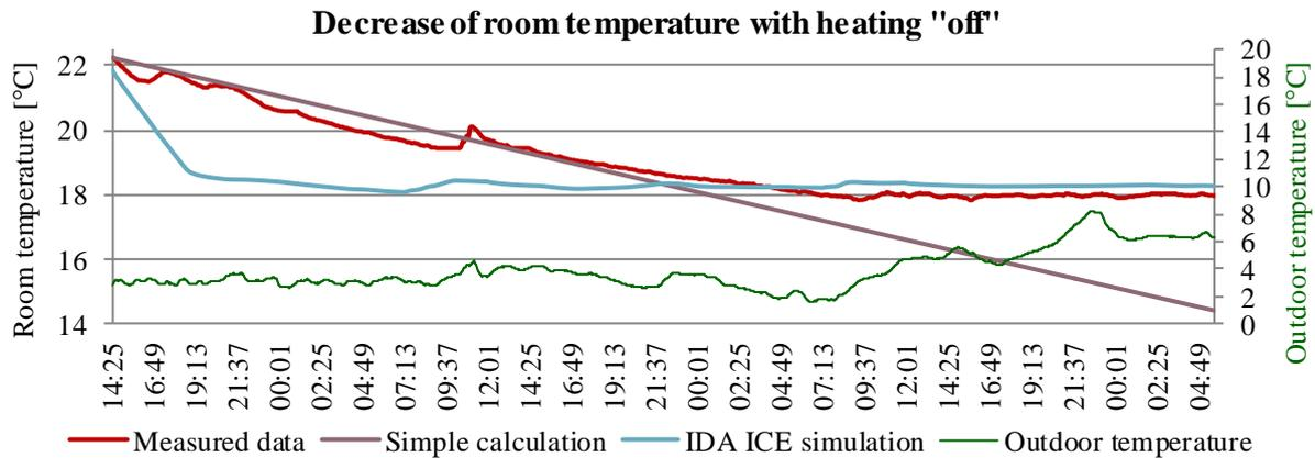
The simulation shows that there is a very fast drop of operative temperature during the first hour after the heating is turned off. However, the temperature for the rest of the weekend drops very slowly, and stabilizes at around 18°C. In order to find out if this occurs due to internal gains in the simulation, a heat balance from IDA ICE is analyzed (see graph below).
