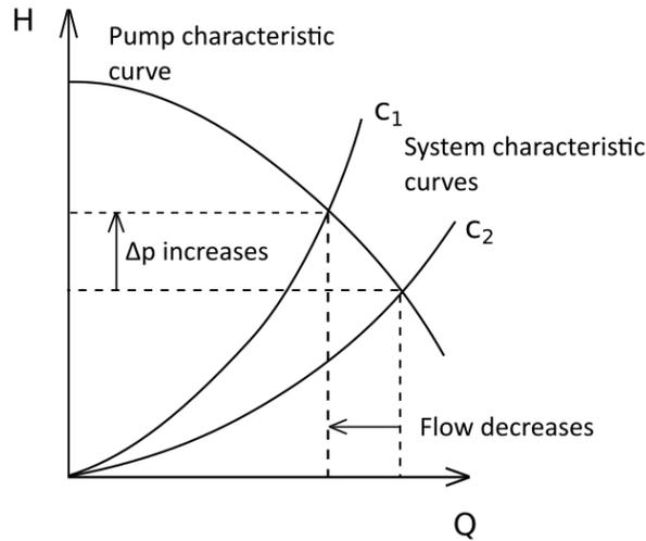
Figure 2.10 Pump with a constant speed regulation: less flow in the system creates higher differential pressure
