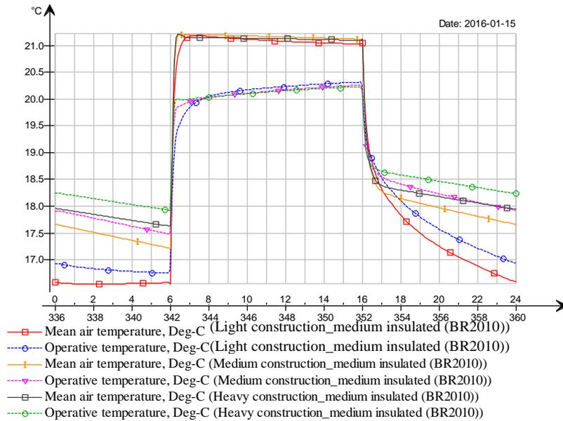
Graph 2.9 Indoor temperatures for light, medium, heavy buildings with insulation level (BR2010)
