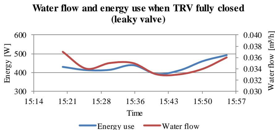
Graph 3.14 Water flow and energy use, leaky valve (window open)
