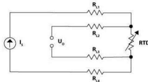
Figure 3.23 4-wire configuration
