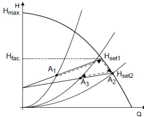
Figure 3.8 Auto adapt mode of the circulation pump, (Grundfos 2016b)
