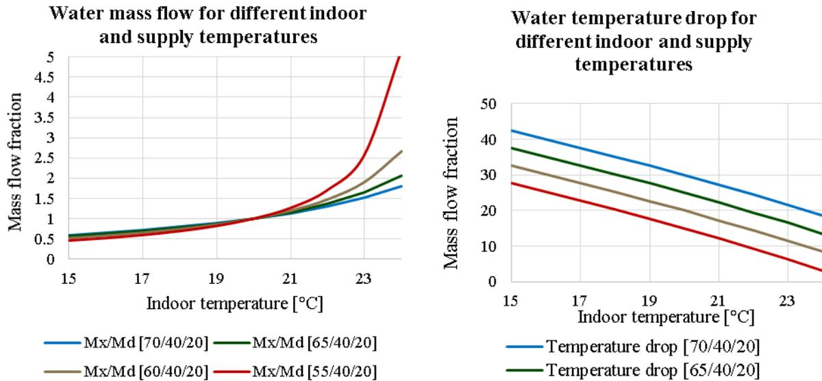
The graphs presented above are the result of the calculation, where the return temperature is fixed at 40°C. Therefore, when decreasing the supply temperature the temperature drop decreases, and the lower the supply temperature the higher the mass flow will be.
