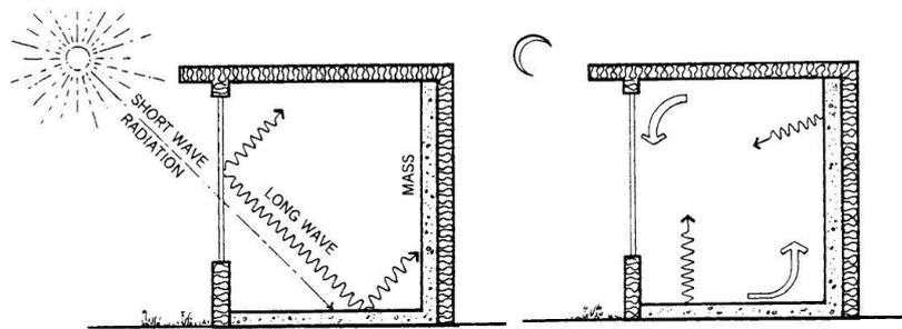
Figure 5.1 Solar radiation, heat storage principle, (Lechner 2015)
