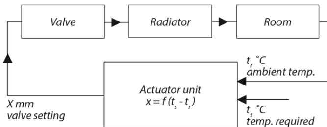
Figure 2.8 Operating principles of thermostats (Danfoss 2010)
