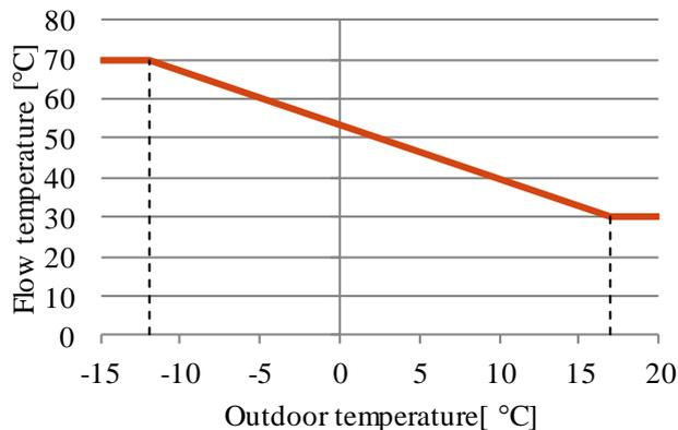
Graph 2.1 Simple heat curve. Supply temperature decreases proportionally to the outdoor temperature increase.
