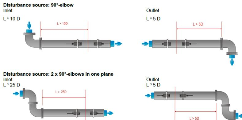
Figure 3.27 Recommended distances from disturbance sources (Katronic Technologies 2016)
