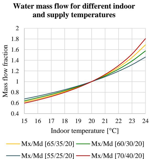
Graph 2.18 Water mass flow for different indoor and supply temperatures
