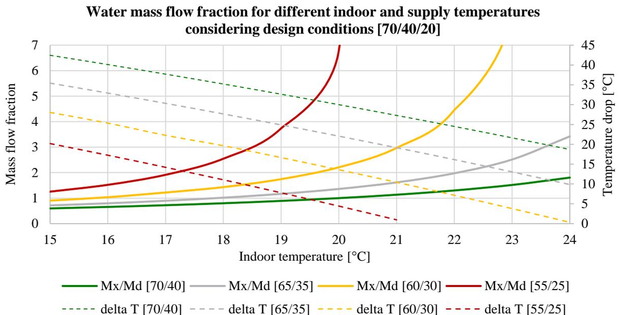
Graph 2.17 Water mass flow fraction for different indoor and supply temperatures considering design conditions [70/40/20]
