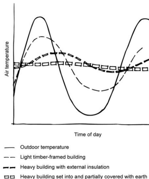
Graph 2.5 Temperature fluctuations for different type of constructions (YourHome, 2013)
