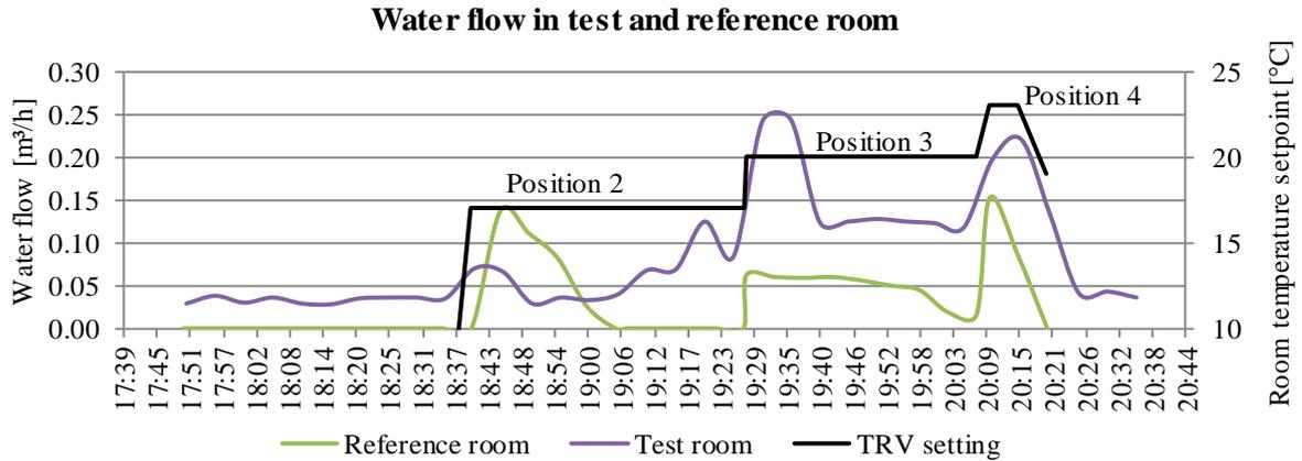
Graph 3.10 Resulting water flow of both meters in test and reference room
