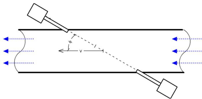
Figure 2.4 The time of flight ultrasonic flow meter, (Engineering ToolBox 2016)
