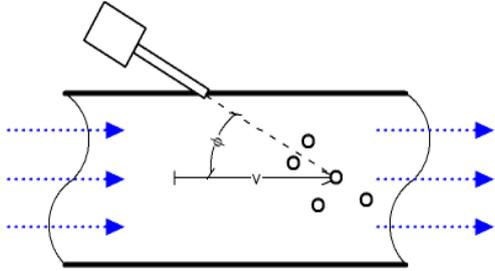
Figure 2.3 The Doppler effect ultrasonic flow meter, (Engineering ToolBox 2016)
