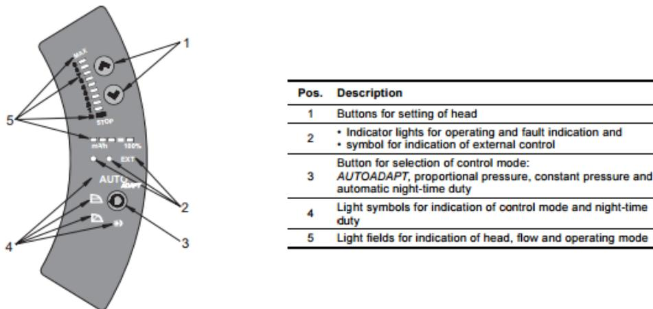
Figure 3.9 Magna 32-120 f control panel, (Grundfos 2016b)
