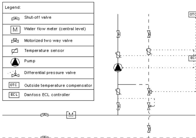
Figure 3.7 Schematic diagram of district heating connection for ground floor of the East block
