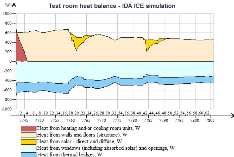
The heat balance from the simulation shows that there was no heating during the whole period, when the room temperature was kept at 18°C. Nevertheless, there are other internal gains that can contribute to the room temperature being so stable over the weekend. The heat accumulated in the internal thermal mass of the room accounts for around 450W according to the simulation; solar gains occur during both days of the weekend.
