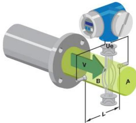
Figure 2.5 Magnetic flow meter, (Instrumentation tools 2016)
