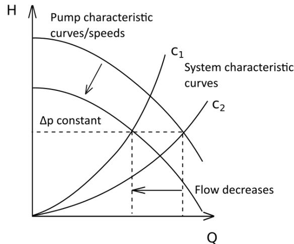
Figure 2.11 Pump with a constant pressure regulation: pressure is not increasing when the flow is decreasing
