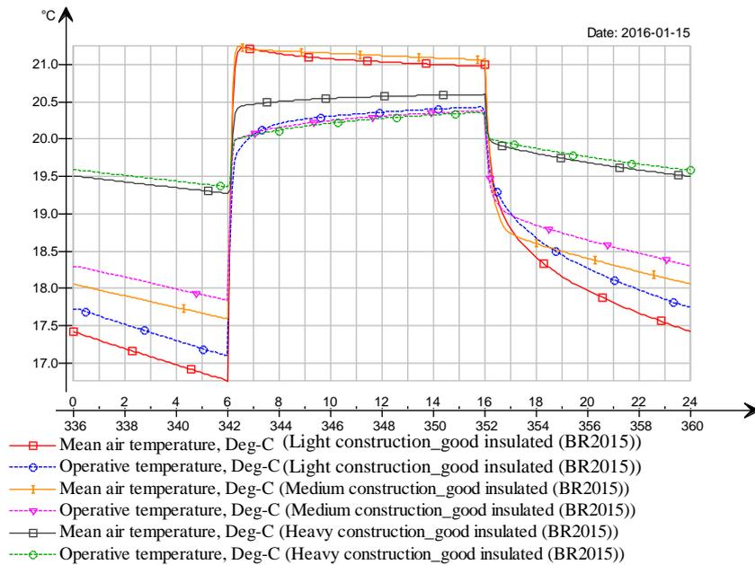
Graph 2.8 Indoor temperatures for light, medium, heavy buildings with insulation level (BR2015)
