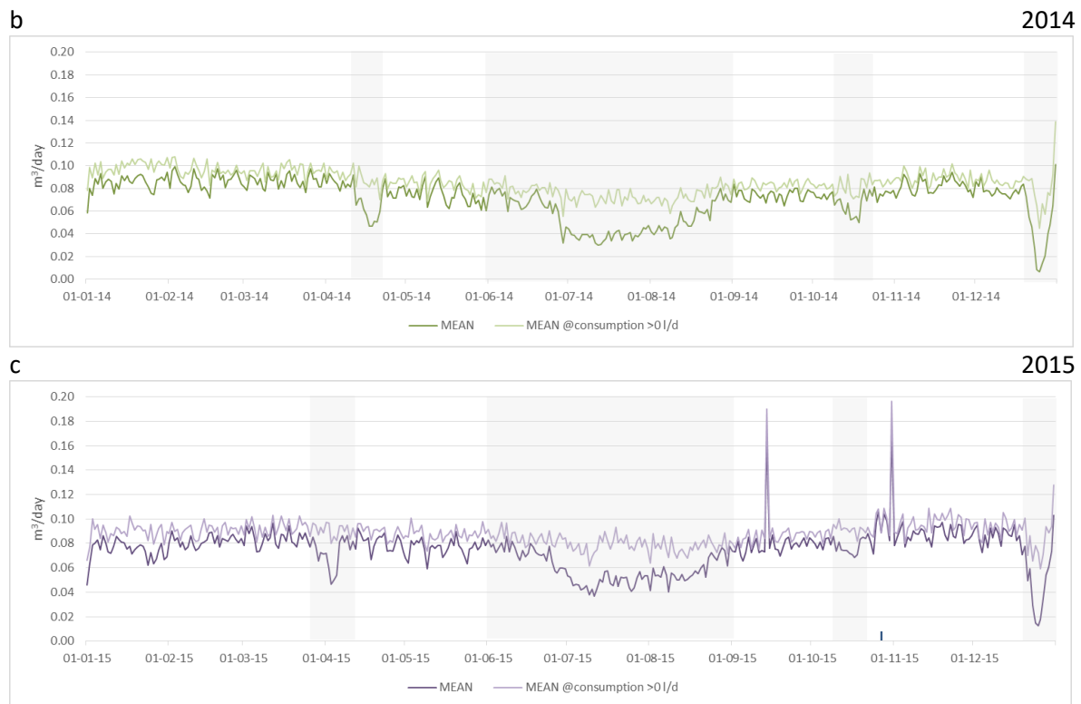
GRAPH 4.8 COMPARISON BETWEEN AVERAGE DAILY HOT WATER CONSUMPTION BASED ON THE WHOLE DATA SET VS. USE HIGHER THAN 0 M 3 /DAY
