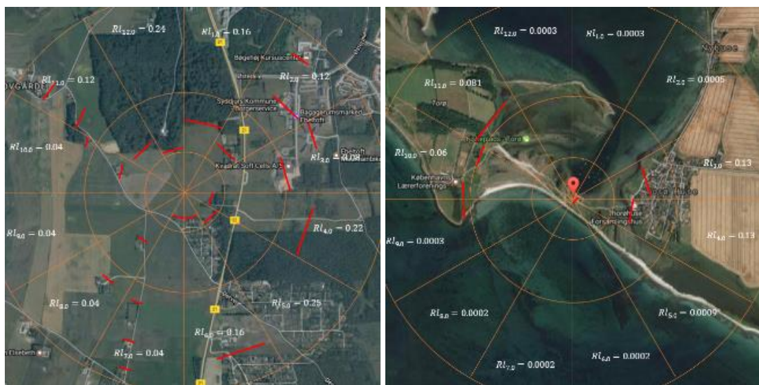
Figure 9.8 – Obstacles at Ebeltoft and Assens implemented in the calculation
