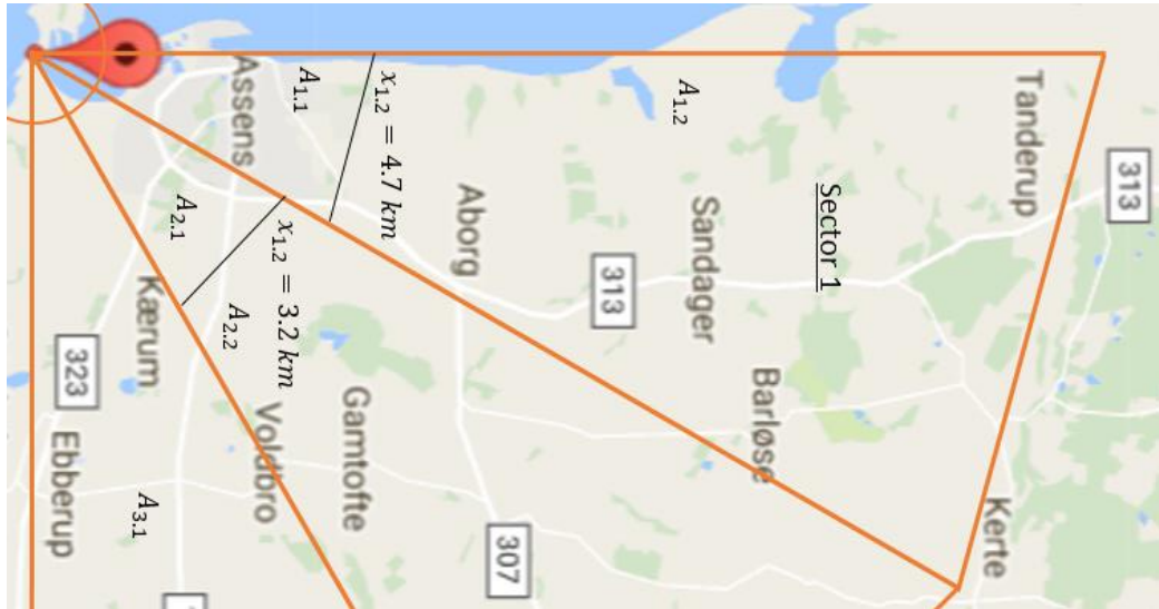
Figure 18.13 – Sector 1, 2 and 3 of roughness rose around DMI measurement station in Assens
