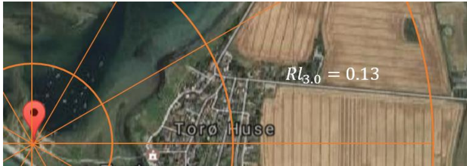
Figure 18.14 – Mean roughness length calculation for Sector 3 at Assens
