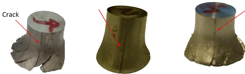
(a) Projectile #5 - Steel. A straight crack in the longitudinal direction. In this case, it initiate from another crack.
