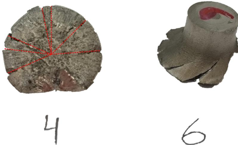
(a) Projectile #4 - Steel. Strike face. Guidelines implemented to help track the cracks, which indicate radial stresses. The cracks are slightly curved, like a helix, into the material, which indicate the cracks are not developed purely by radial stresses.
