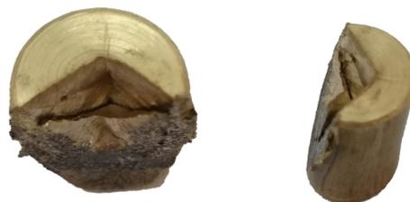
(b) Brass - Impact velocity: 214,7 m/s. Top view.
