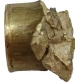
Figure 5.10: *Brass - Impact velocity: 282,0 m/s. Complete projectile defeat, and no pattern in the fracture planes.*
