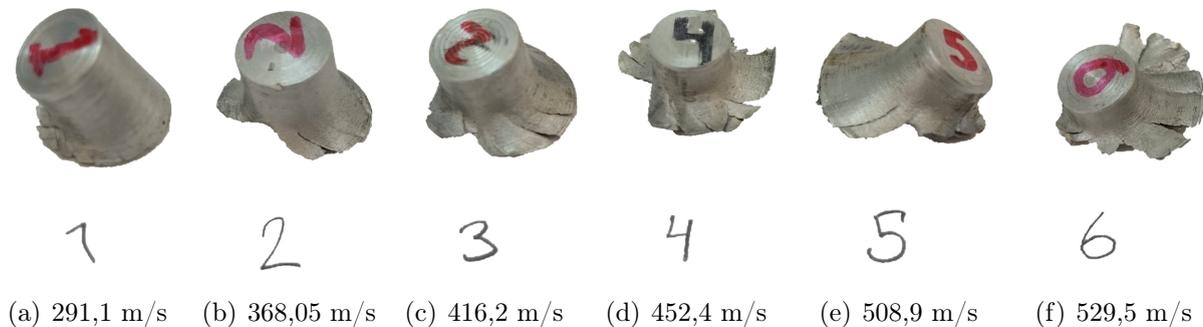
Figure 5.5: *Aluminium projectiles following impact on 12 mm ARMOX 500 plate.*
