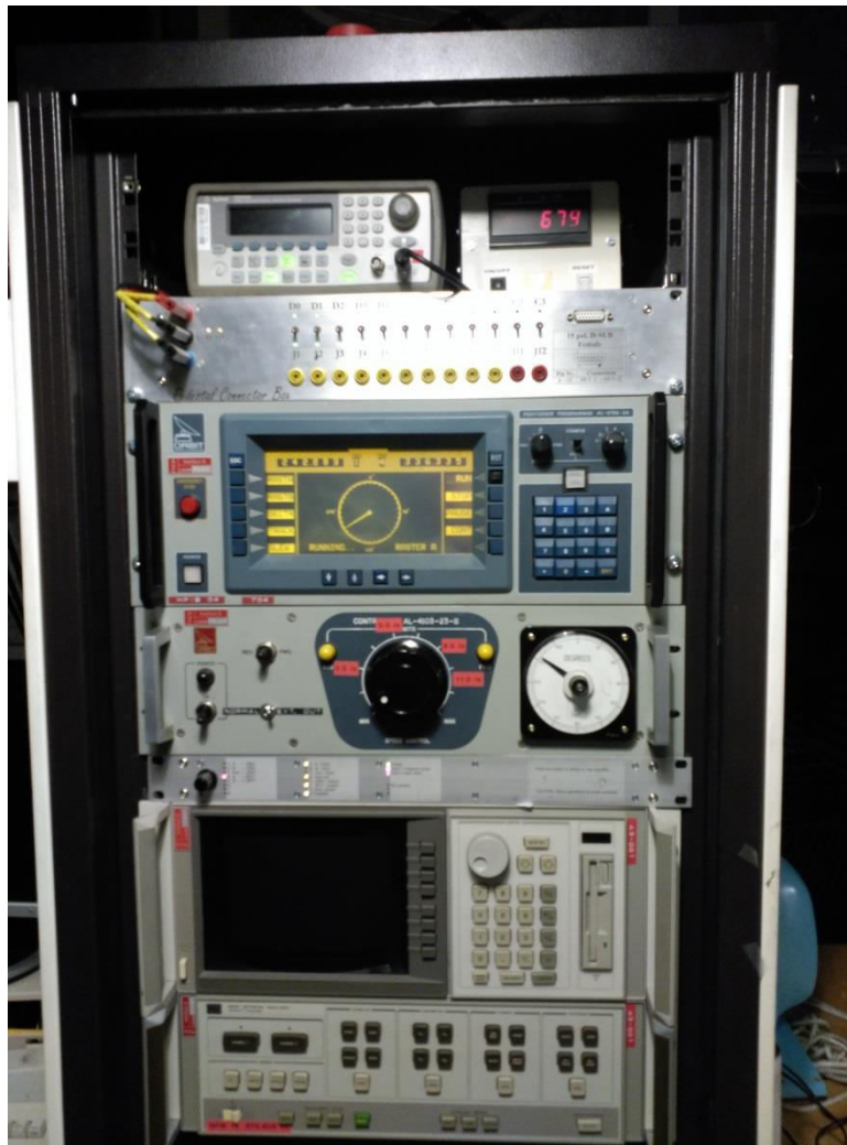
Figure 4.33: Picture of the device used to control the movement of the pedestals in the anechoic chamber.
