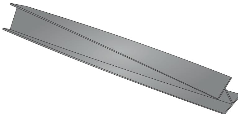
**Figure 1.1:** St. Venant/Homogeneous torsion
