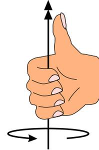
**Figure 2.2:** Right-hand rule applied to define the positive moment and rotation directions.
