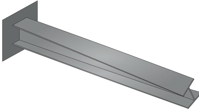
**Figure 1.2:** Vlasov/Non-homogeneous torsion
