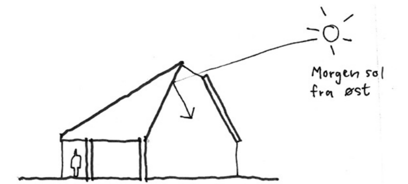
III.06.07 The skylight catches the morning sun
