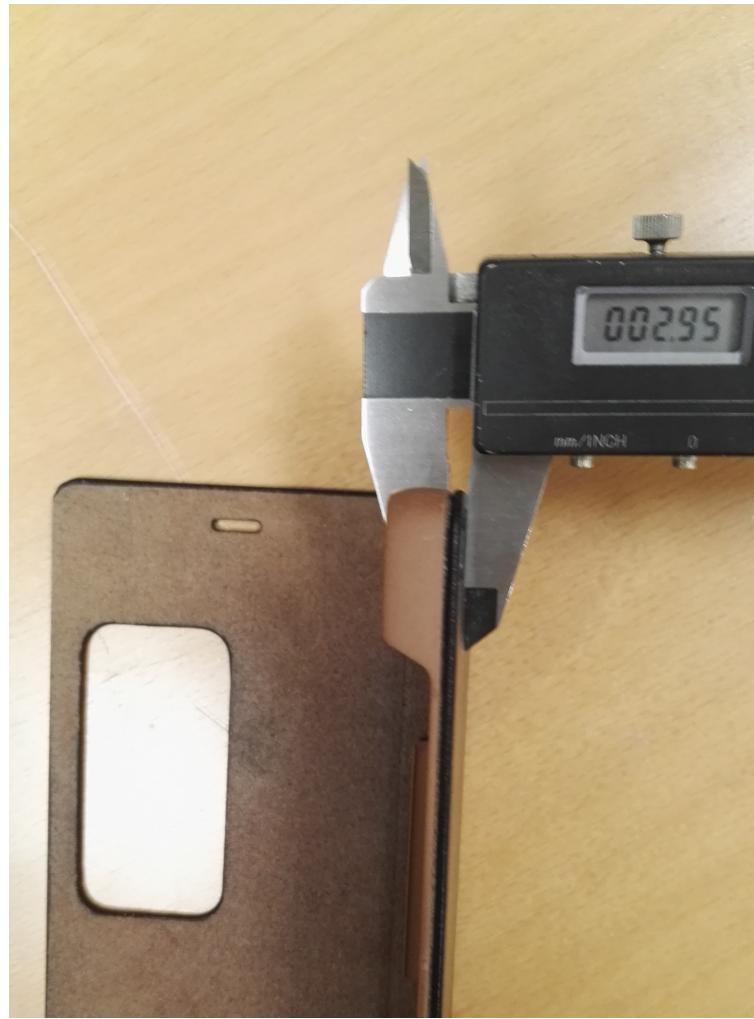
Figure A.2: Width of bottom of the cover
