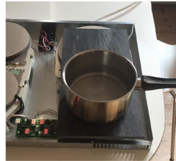
ILL. 53: TESTING INDUCTION WITH A SLATE PLATE
