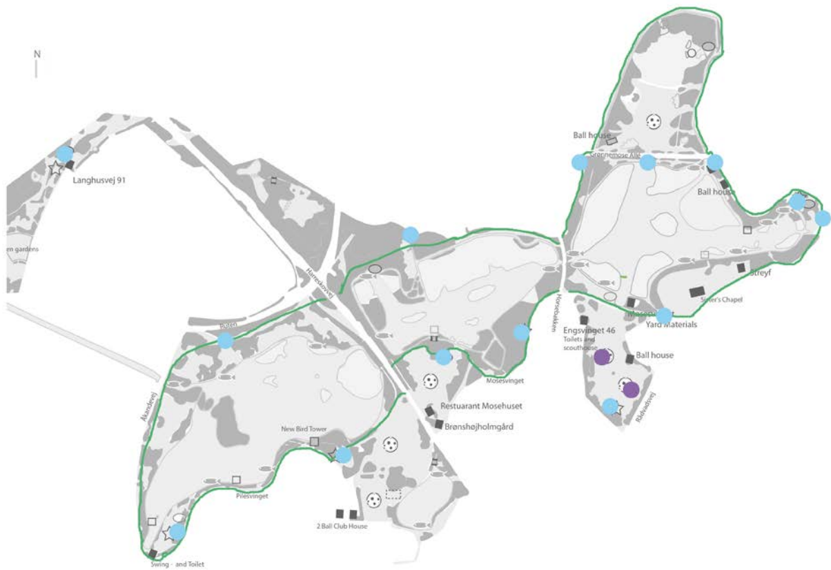
Figure 57. Position of luminaries.
