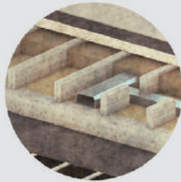
Close up. Ventilation in the floor
