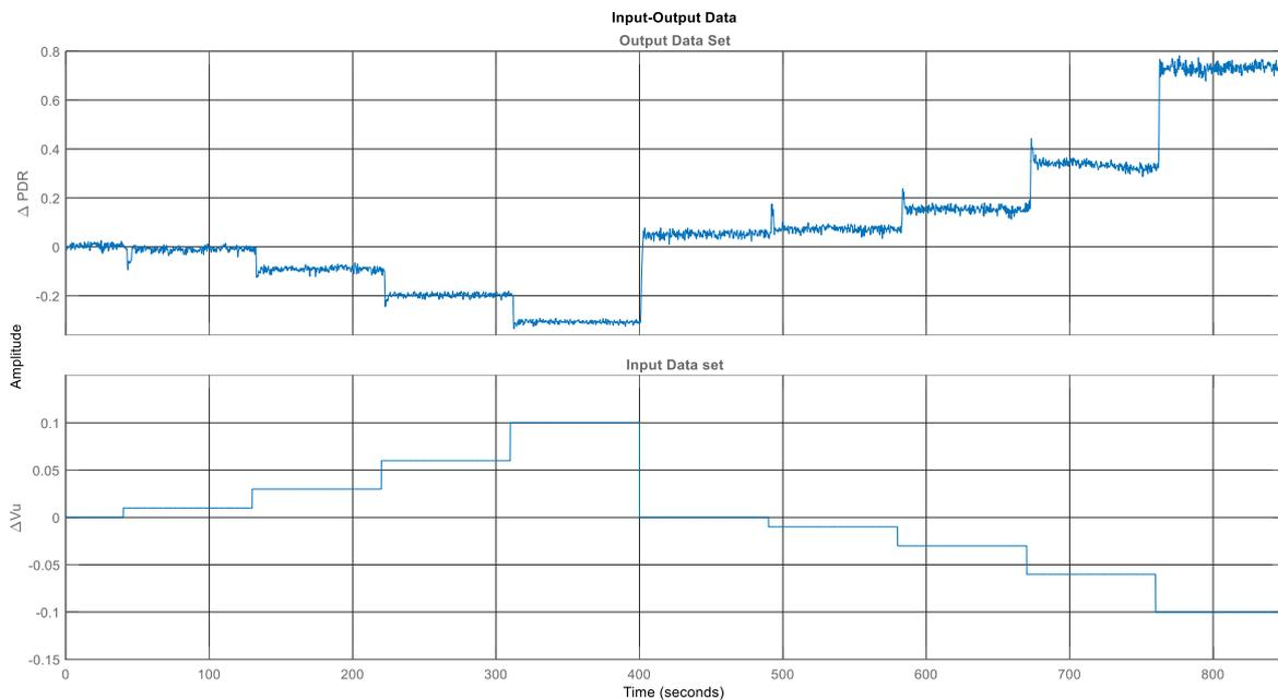
Fig. IV.2 Underflow valve identification data set.
