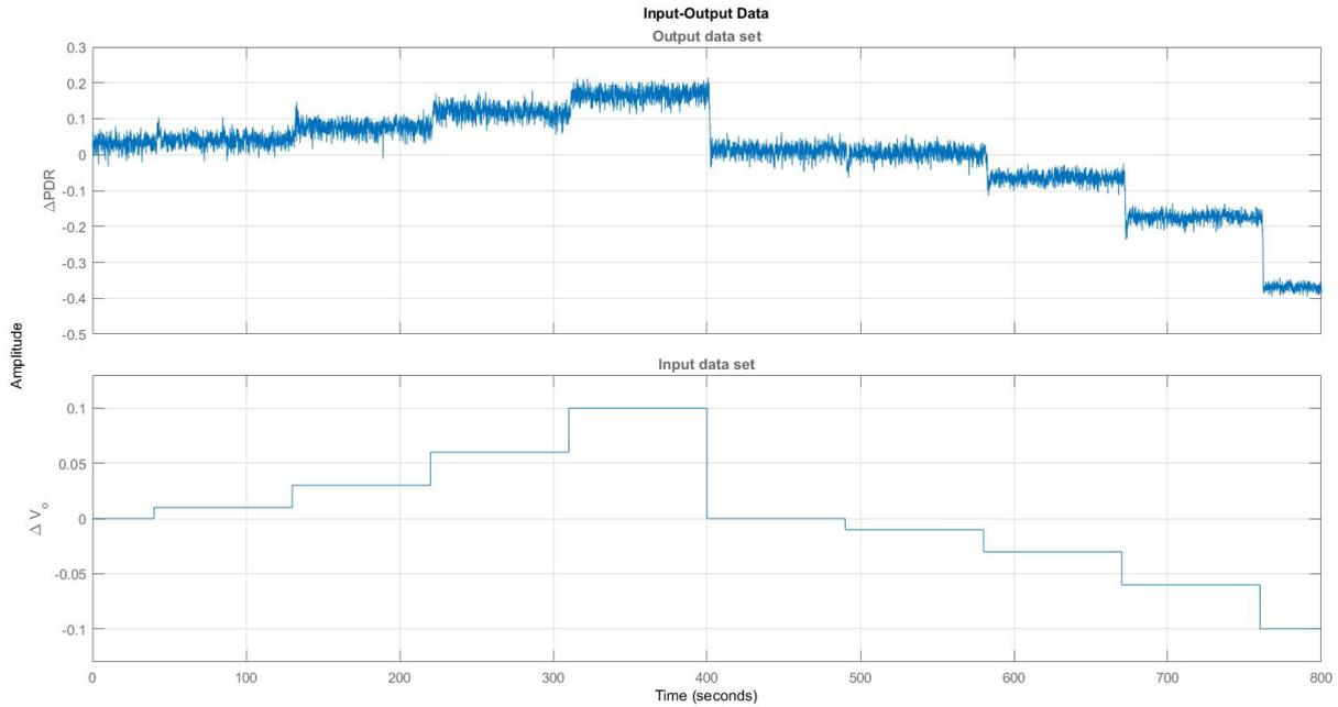
*Fig. IV.7 Underflow valve model identification data set.*
