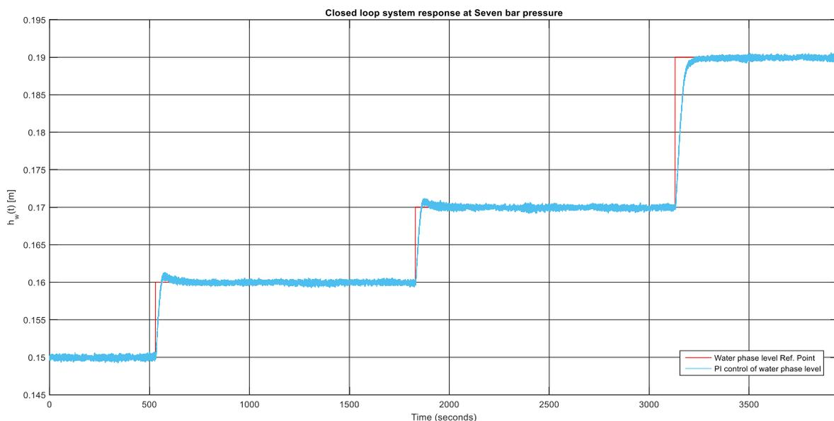
Fig. III.5 Closed loop system response at Seven bar pressure
