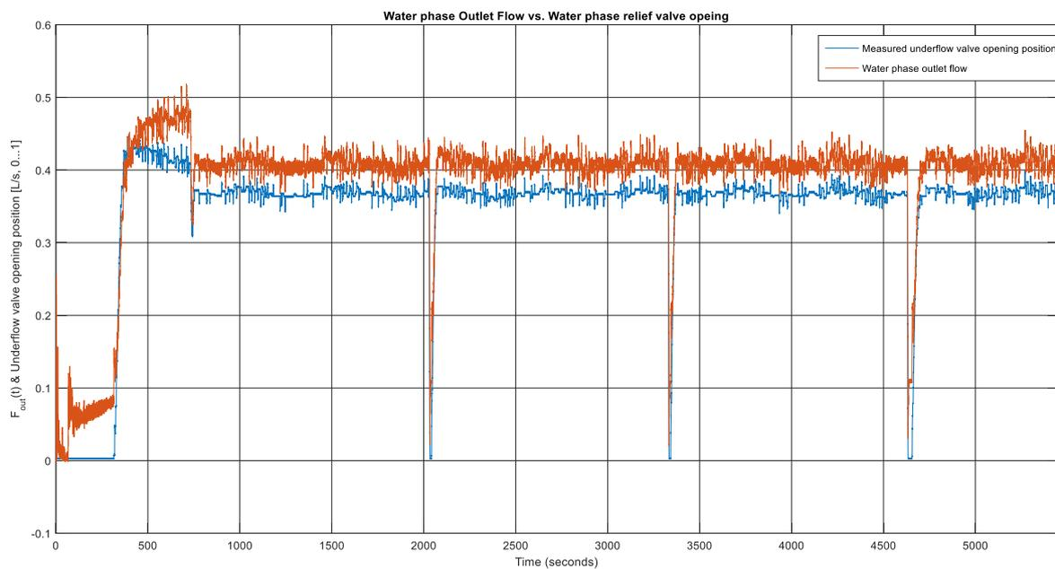
*Fig. III.6 Water phase outlet flow vs. Water phase relief valve opening.*
