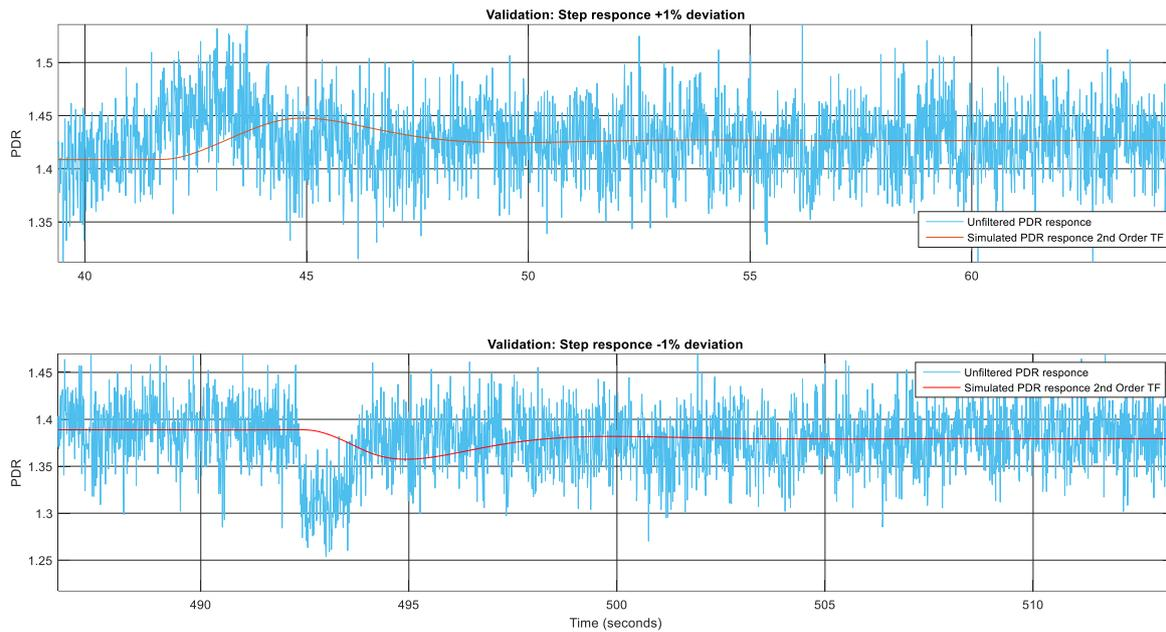
*Fig. IV.10 Step response for one percent deviation in valve opening position.*
