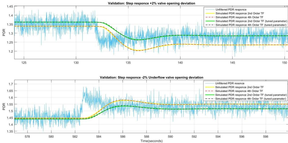
Fig. IV.6 Step response for two percent deviation in valve opening position .
