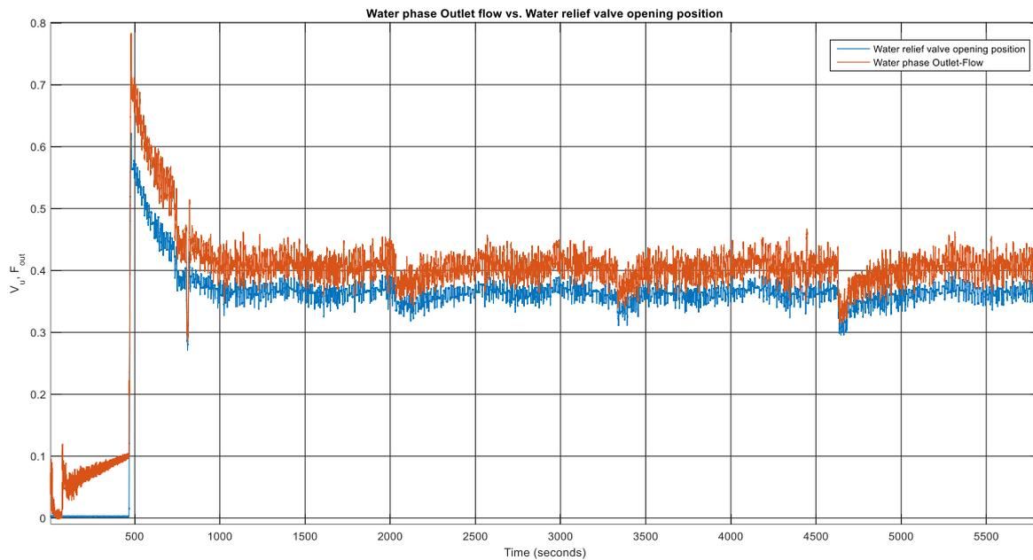
Fig. III.17 Water phase relief valve opening vs. Outlet flow.
