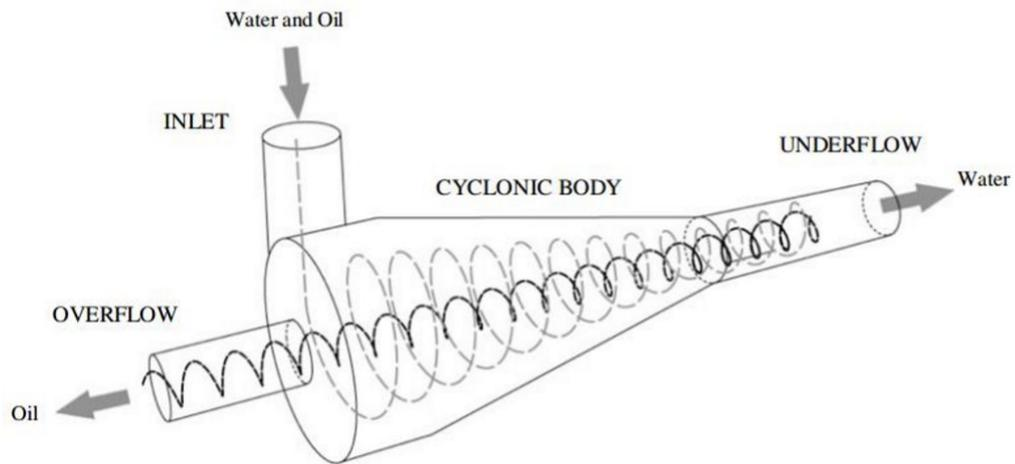
*Fig. I.2 Hydro-cyclone separator [1, 2]*
