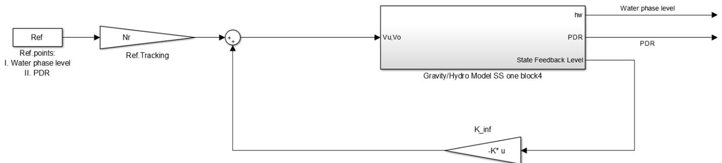
Fig. VI.1 MIMO LQR control structure.
