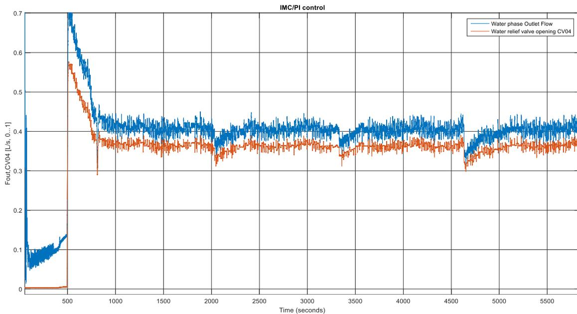
*Fig. III.12 Water phase relief valve opening vs. Outlet flow.*
