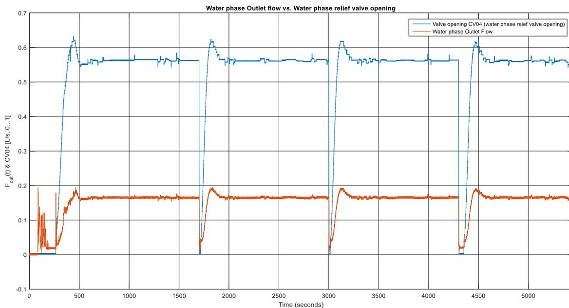
Fig. III.4 Underflow valve opening position vs. Water phase Outlet flow.
