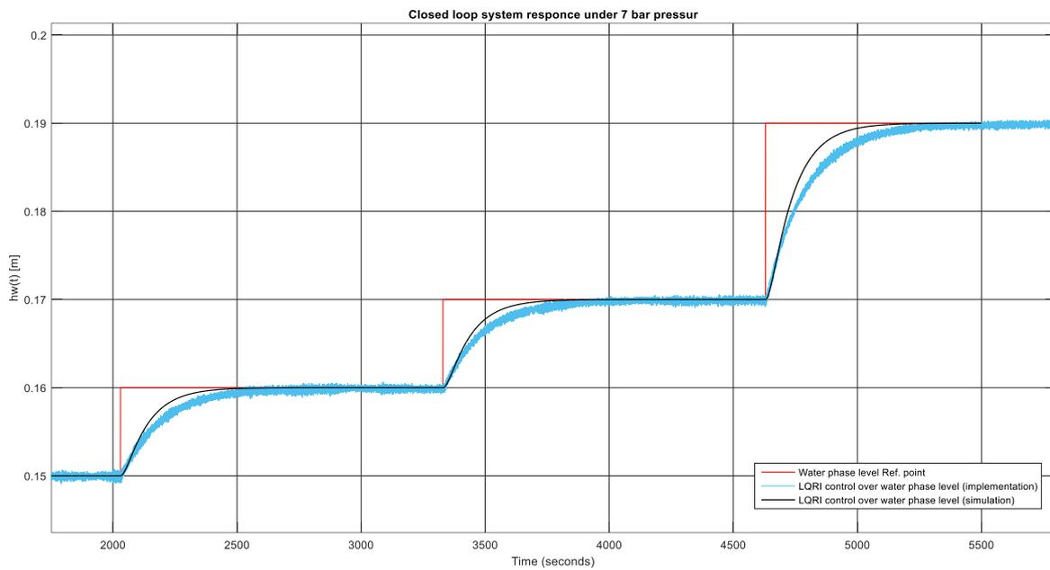
*Fig. III.16 Closed loop system response with LQRI control.*
