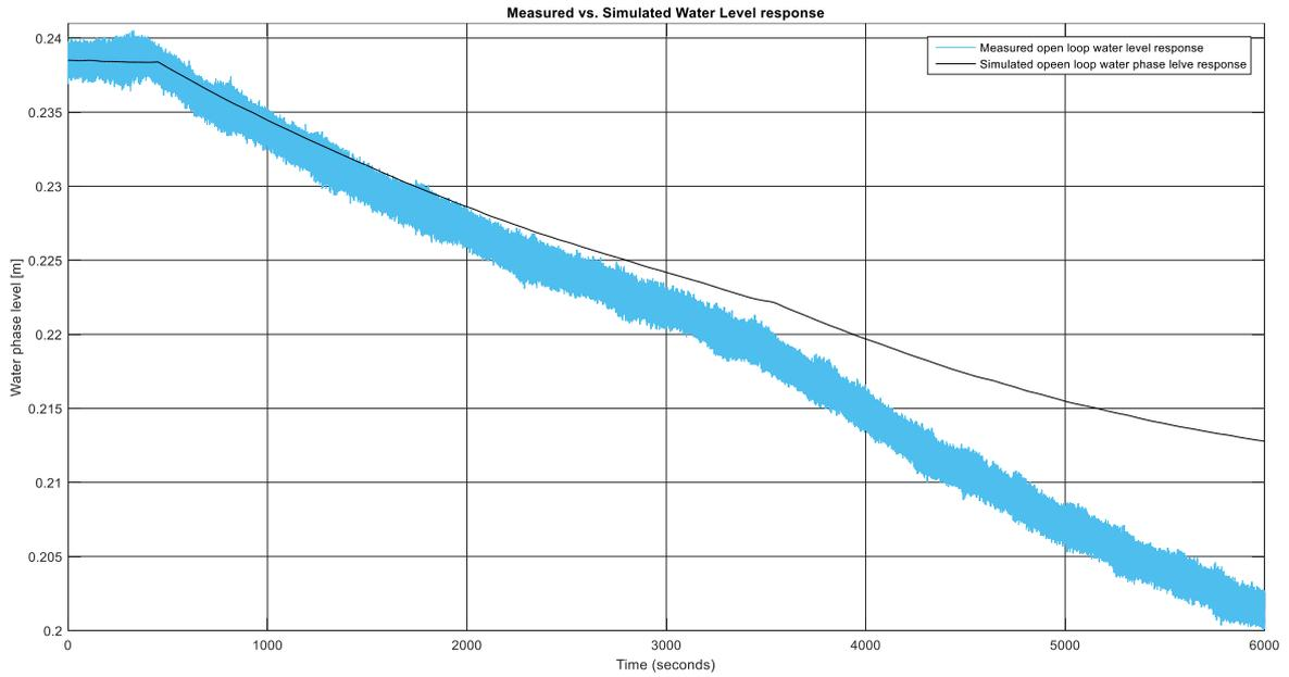
Fig. II.2 Nonlinear model validation for water phase level
