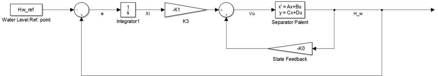
Fig. III.15 Closed loop system with integral control.
