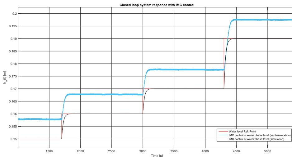
Fig. III.8 Closed loop system response with IMC control.
