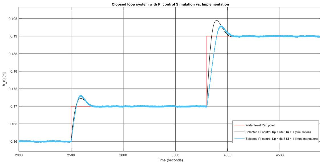
Fig. III.3 Closed loop Simulation vs. Implementation, one to two percent step increase.
