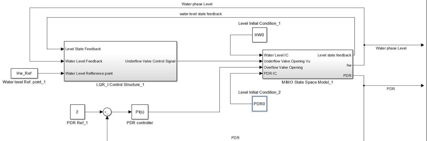
Fig. V.4 Closed loop MIMO system.
