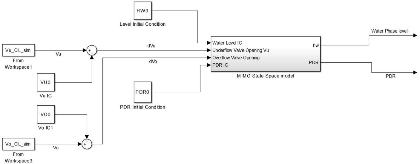
Fig. V.1 MIMO state space simulation model.
