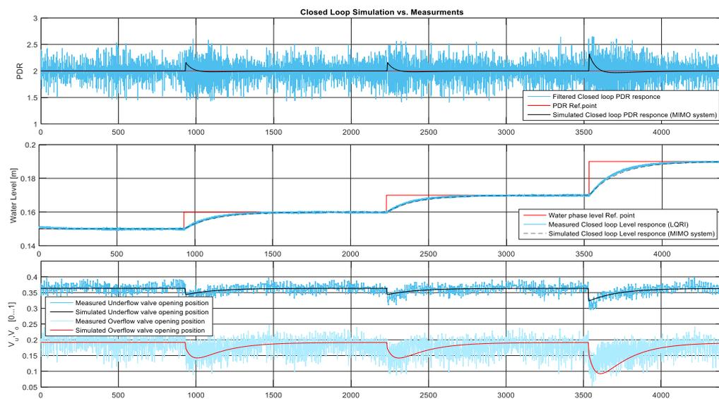
Fig. V.5 Closed loop MIMO validation.
