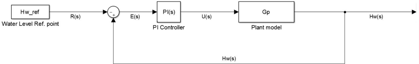
Fig. III.1 Closed loop system with PI control structure
