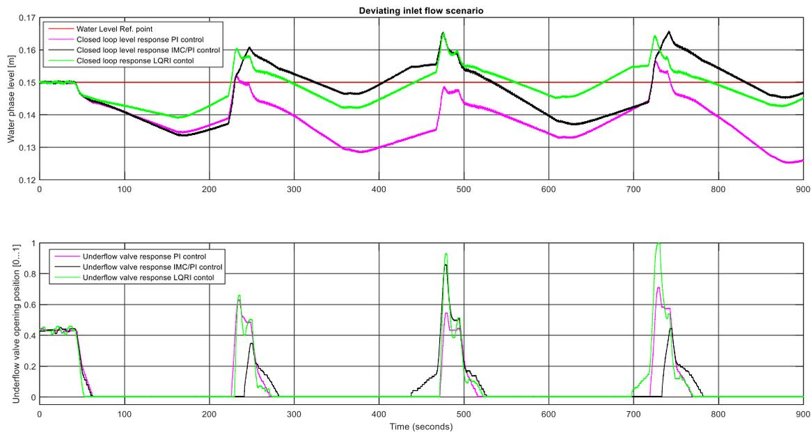
Fig. III.19 Closed loop response under worst case scenario.
