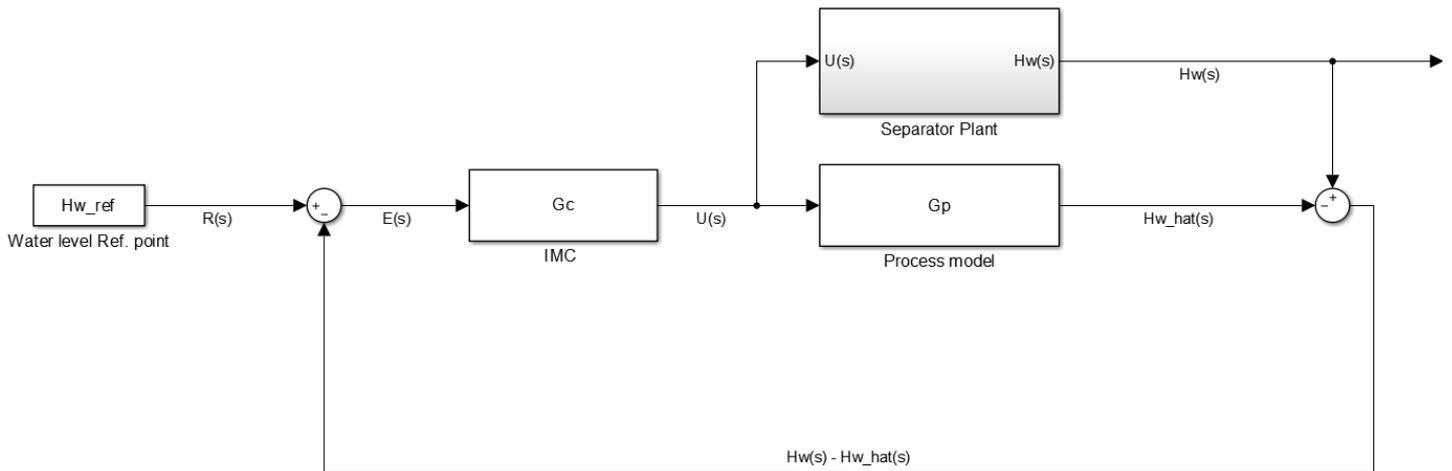
Fig. III.7 Closed loop system with IMC control structure.
