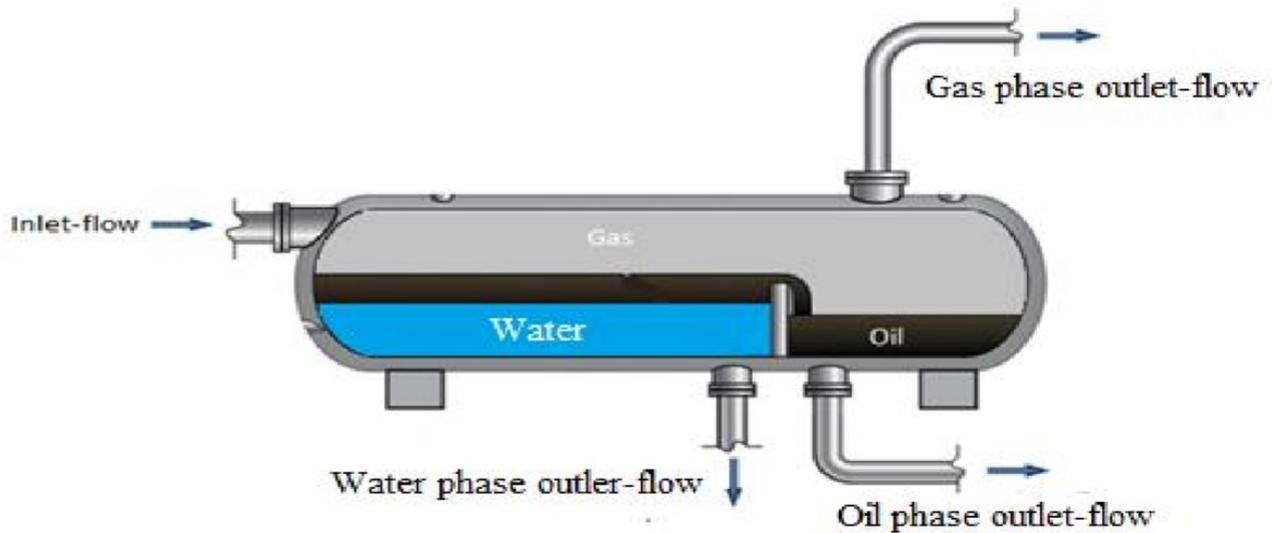
Fig. I.1 Three phase gravity separator system [ <http://goo.gl/fymPiv> ]
