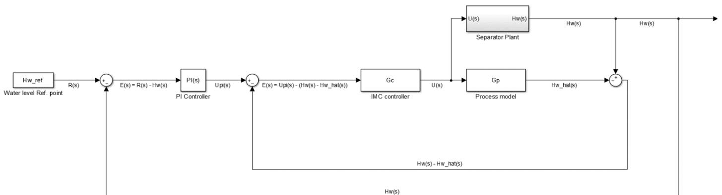
Fig. III.9 IMC/PI control structure
