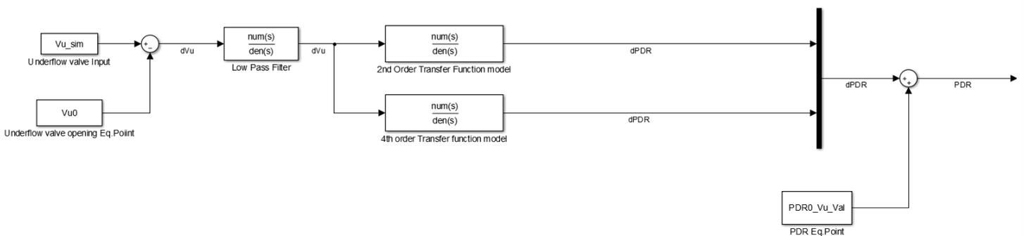
Fig. IV.4 Underflow valve opening position to PDR simulation.
