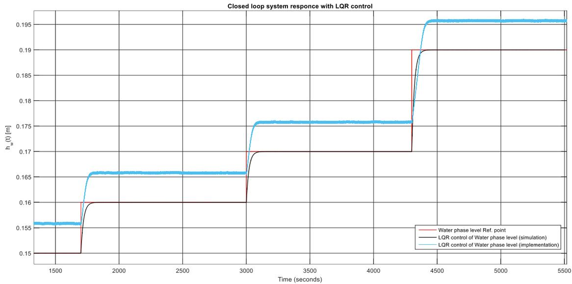
Fig. III.14 Measured vs. Simulated closed loop system response
