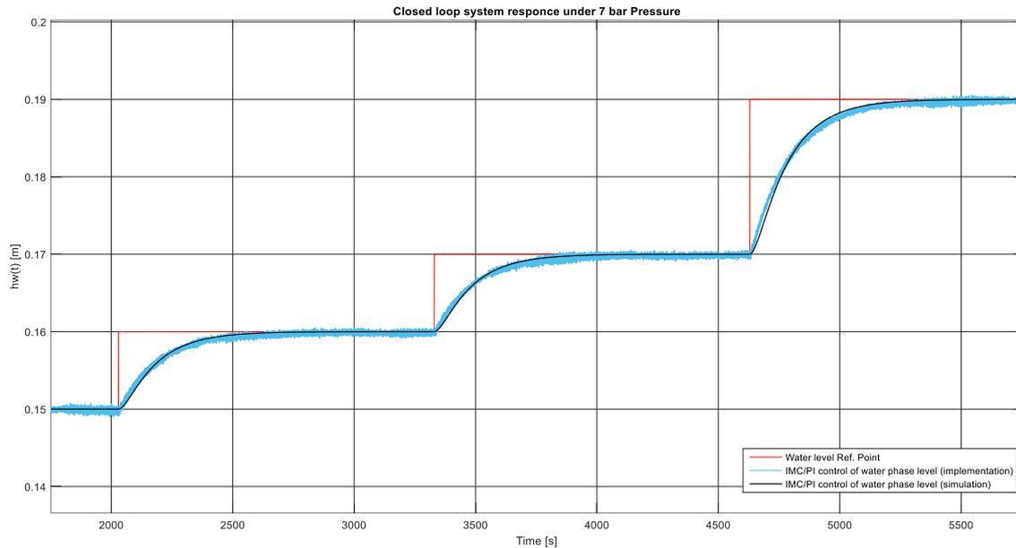
*Fig. III.11 Closed loop system response with IMC/PI control structure.*
