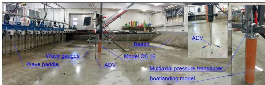
Figure 5.4. Test set up in the basin.
