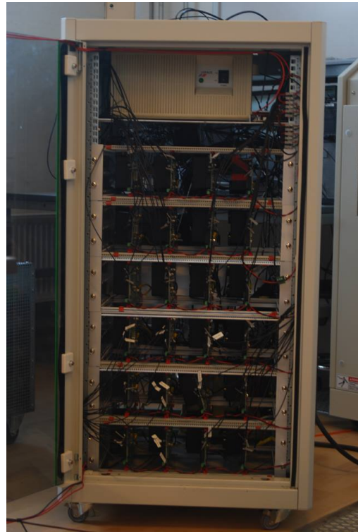
FIGURE 6.1: The MMC prototype with four sub-modules per arm in Aalborg University.
