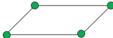
**Figure 6.2:** 4 nodes shell elements.
