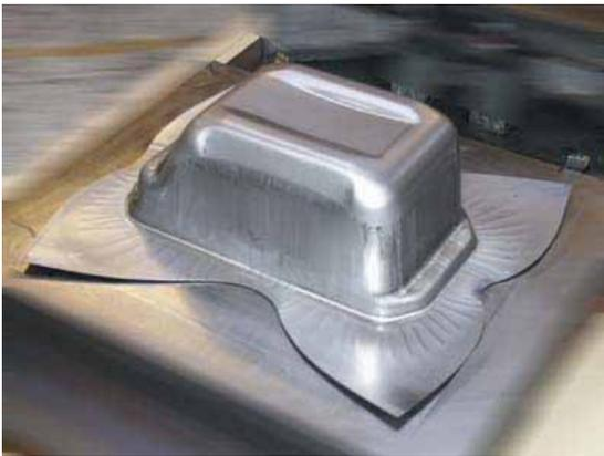
**Figure 3.2:** Illustration of a faulty deep drawing process of a sink.
