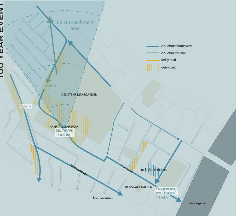
Storm water management diagrams for a 1 year and a 100 year rain event displaying the strategies for run off water managed in surface solutions.
