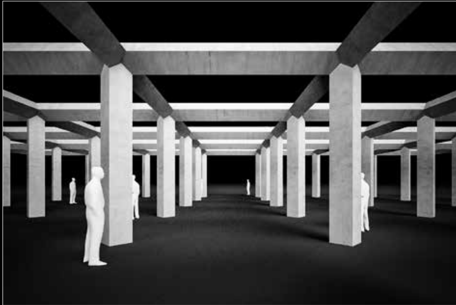
0,8m thick columns with 5,6m in between from center to center
