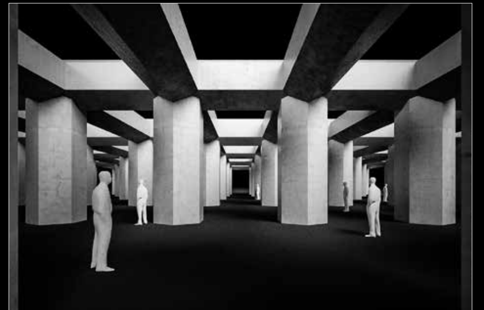
1,6m thick columns with 5m span in X direction, and 10m span in Y direction.
