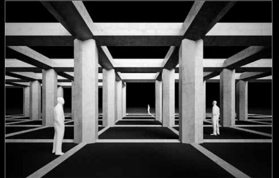
0,8m thick columns with 3,6m in between from center to center
