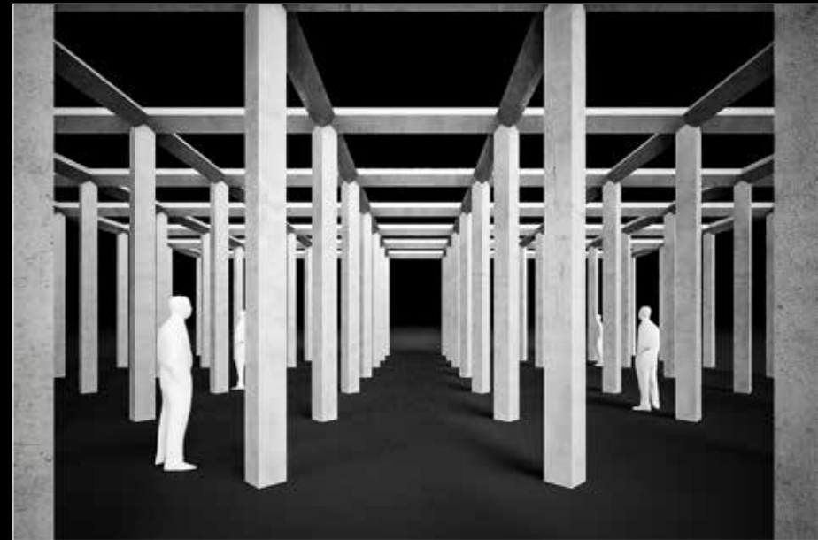
0,4m thick columns with 2,8m in between from center to center
