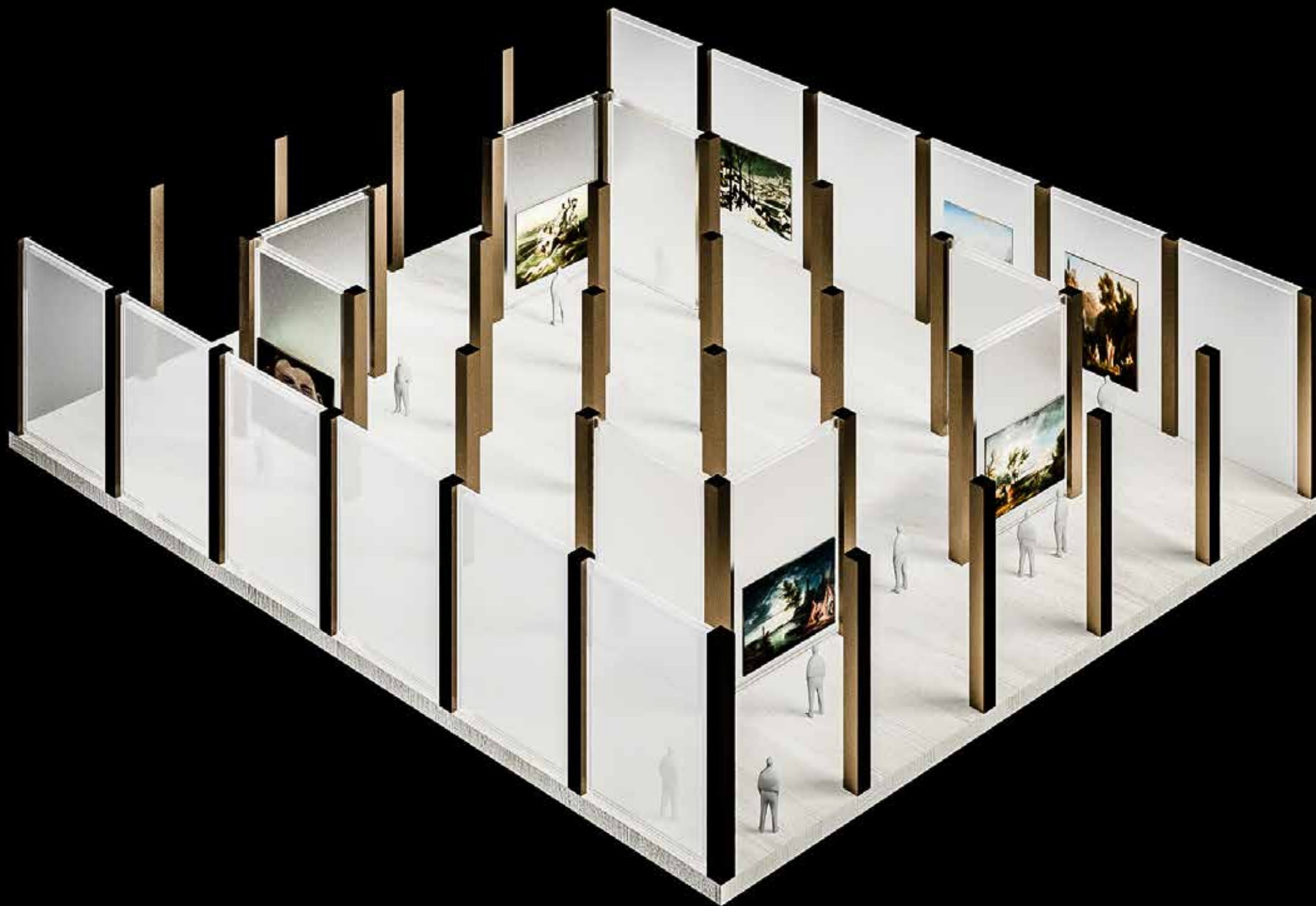
GREY ASH SONOMA OAK FLOOR FROSTED GLASS PARTITION WALLS (INNER) / WHITE PLASTER PARTITION WALLS (OUTER) BRASS CLAD CONCRETE COLUMNS
