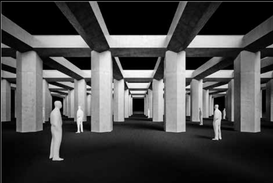
1,6m thick columns with 5m span in X direction, and 10m span in Y direction.
