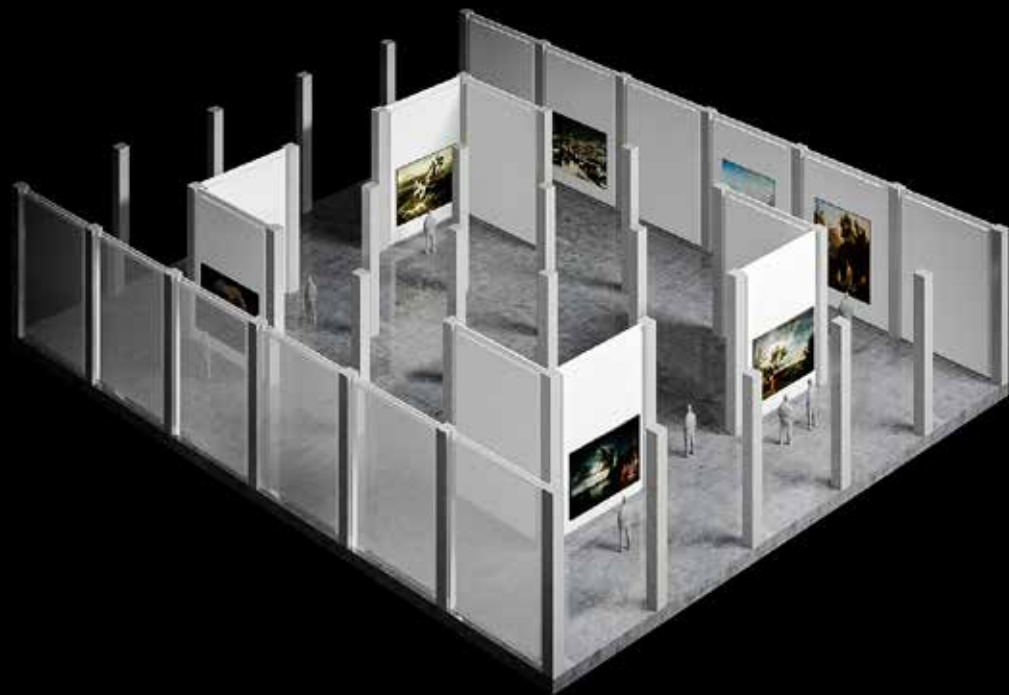
ROUGH GREY CONCRETE FLOOR WHITE PARTITION WALLS GREY CONCRETE COLUMNS
