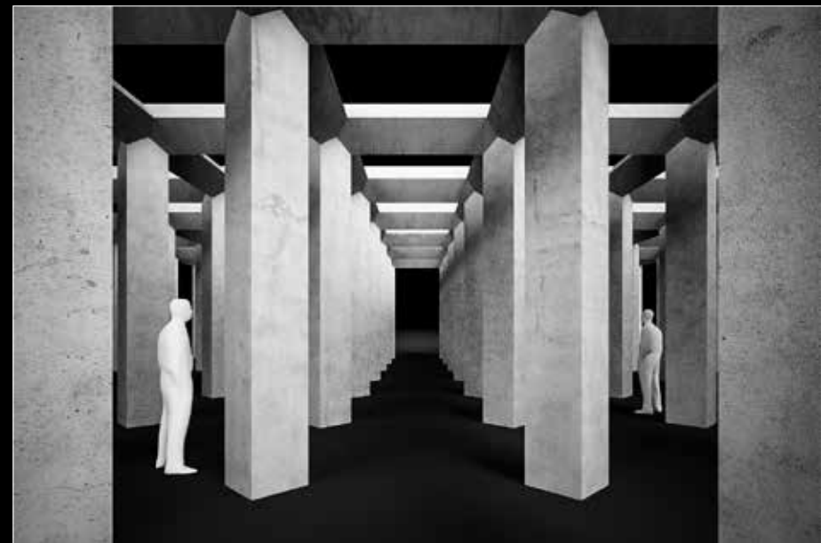
0,8m thick columns with 2,8m in between from center to center
