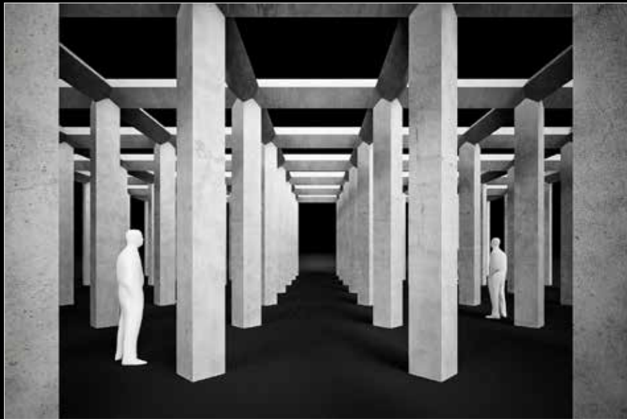
0,6m thick columns with 2,8m in between from center to center
