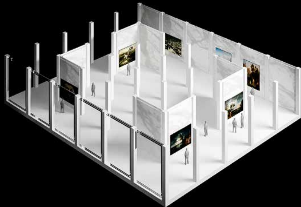
GREY CONCRETE FLOOR MAPLE WOOD PARTITION WALLS GREY CONCRETE COLUMNS
