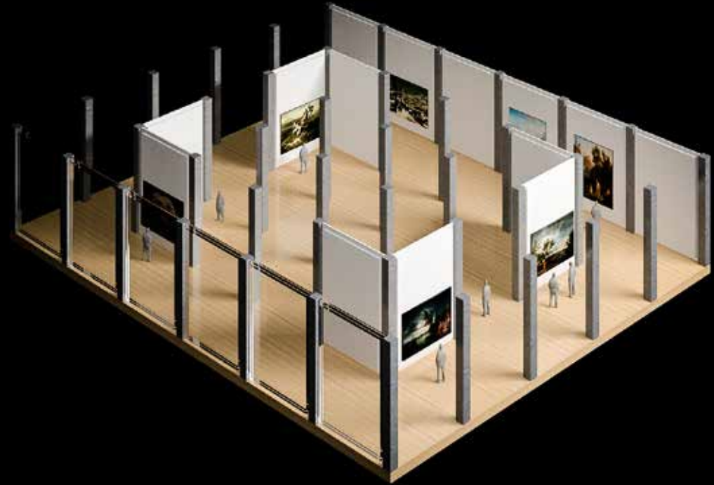
MAPLE WOOD FLOOR WHITE PARTITION WALLS ROUGH GREY CONCRETE COLUMNS
