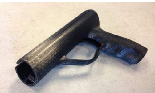
Ill. 3.3.2: 3D-printed model of the speargun handle
