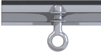
Ill. 3.1.4: Locking mechanism between the two barrels. The spring component locks in holes in the muzzle.
