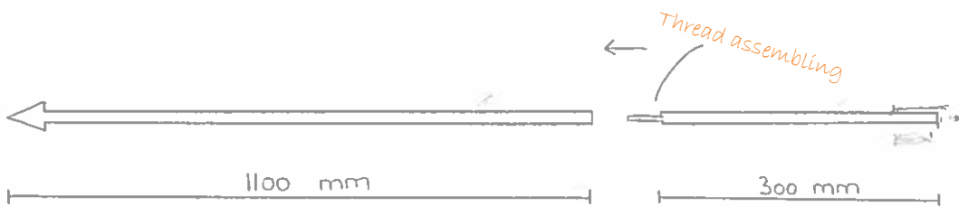
Ill. 2.8.1: Spear sizes for different speargun sizes
