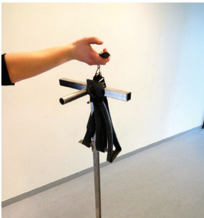
III. C.07: The welded model with bicycle tube as rubberband
