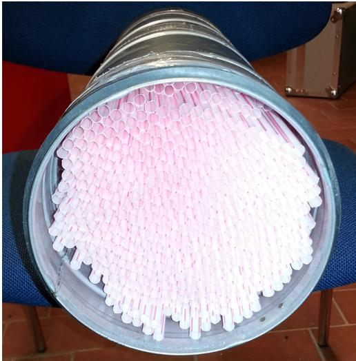
*Figure 6.4.* Duct filled with straws
