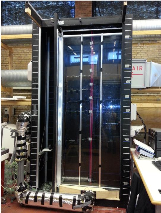
*Figure C.1.* Experimental setup(Hot box)
