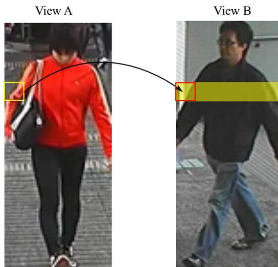
**Figure 3.25:** Matching patches between camera views. Patches in view A are matches with patches at the same horizontal level (yellow area) in view B and the shortest match is returned.
