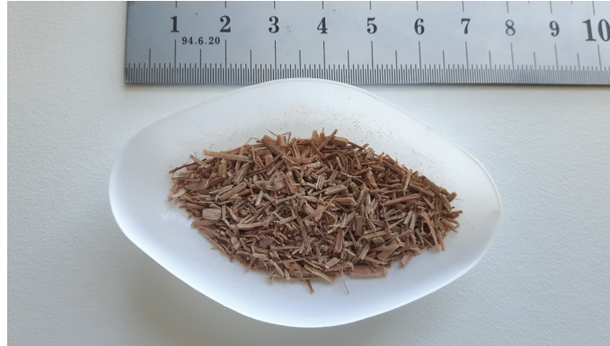
Figure 2.1: Grinded eucalyptus tree used for the tests. The longest of the grinded wood fibers are \approx 6 mm.
