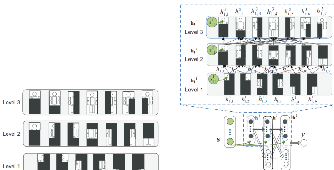
Figure 2.13. The model for visibility reasoning and detection label estimation [Ouyang and Wang, 2013]
