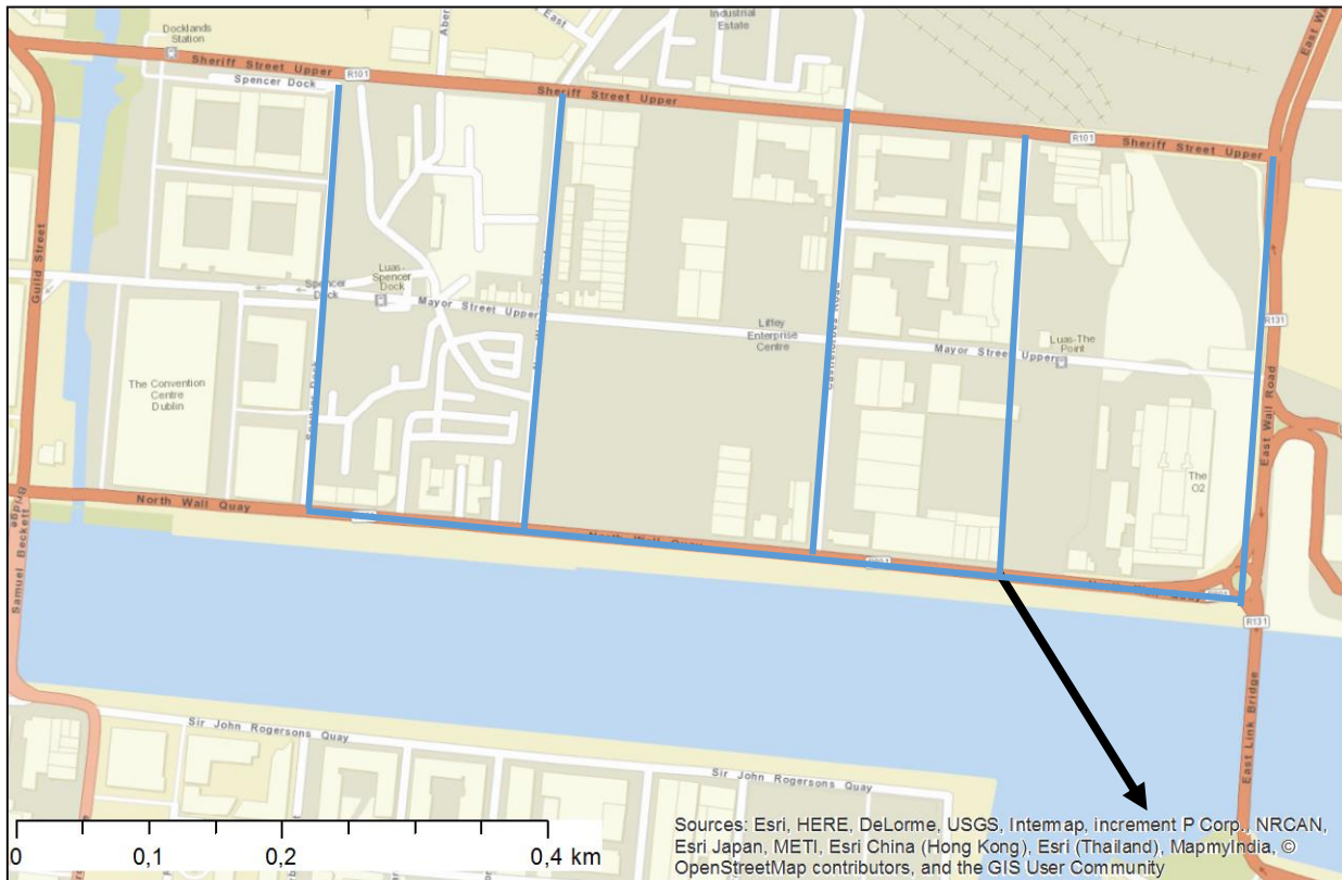
Figure 7-4 The future transmission (black) and distribution (blue) pipes for Spencer Dock
