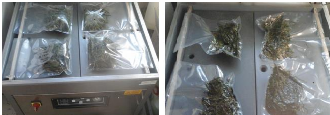
Figure 14. Vacuum packing machine with the bales prior (left picture) and after (right picture) vacuum packaging.
