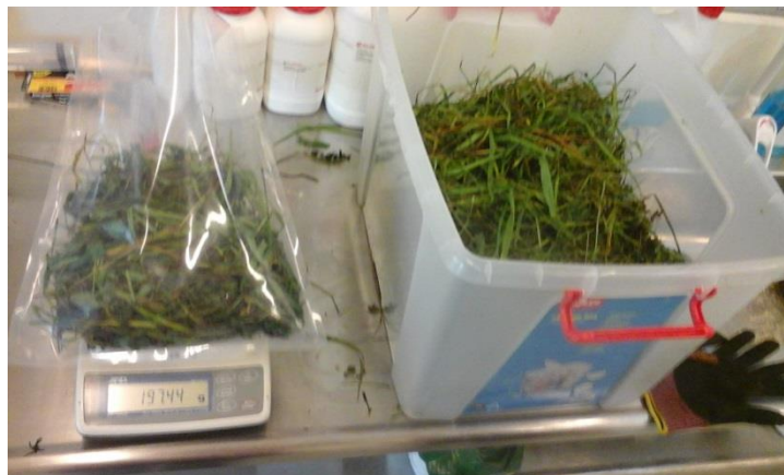
Figure 13. Preparation of silage bags. Around 200 g of fresh material were included in the bag after homogenization in the box on the right.
