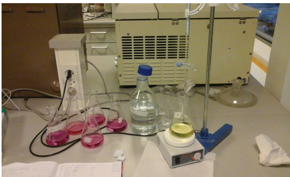
Figure 5. Titration of ammonia during TKN analysis.
