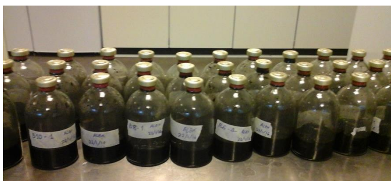
Figure 17. Batch vials containing the biomass and the inoculum.
