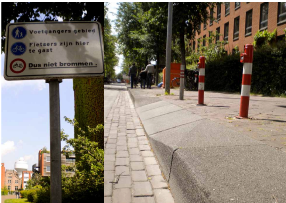
Figure 13: Signposting stating that only non-motorized vehicles are allowed in the area (left) and raised curbs and bollards preventing unauthorized access by vehicles (Foletta & Field, 2011)
