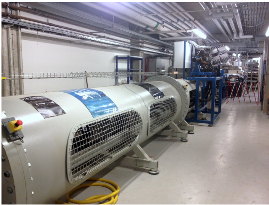
Figure 3.1. The WaveStar PTO test bench.
