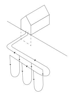
ill. 042-B: Brine to water system producing sustainable heat by using the passive heat storage with the ground.
