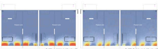
Test of the daylight for facade iteration 1 shows that the daylight nearly illuminates the whole patient unit, but it comes at the cost of high amounts of solar radiation that cause overheating as seen on illustration ??
