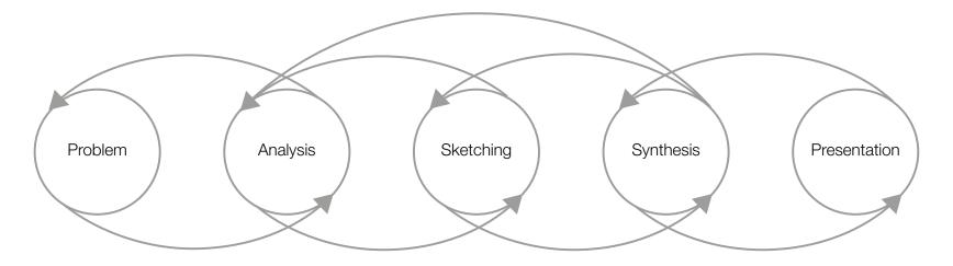
ill. 001: Diagram showing the relation between each phase of the integrated design process (Knudstrup, 2005)
