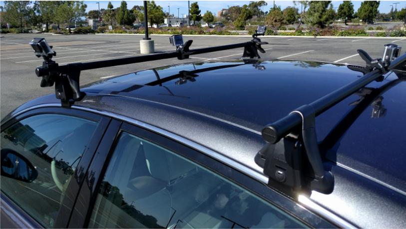
**Fig. 5.1:** Configuration of four GoPros mounted on the test vehicle to achieve a full surround view.
