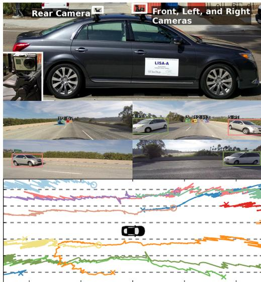
Fig. 1. Vehicle instrumented with four cameras (top), ground truth bounding boxes in the four perspectives (middle), and 3D ground truth trajectories (bottom).
