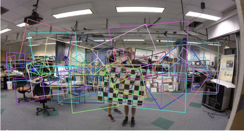
Fig. 5.3: Checkerboard distribution used to calibrate the intrinsic parameters of the GoPro.
