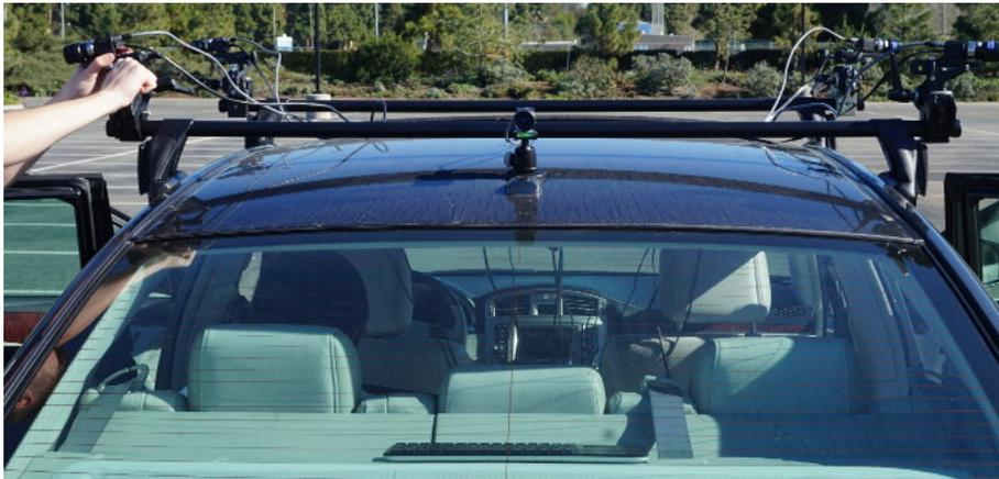
(d) Sixcam setup. The front perspective is located inside the cabin.
