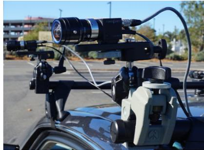
(b) Side view camera with wide-angle lens
