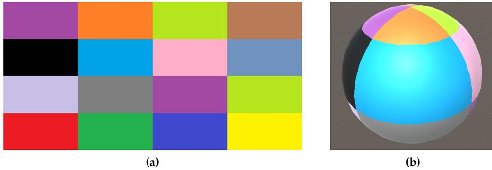
**Figure 2.16:** Projection in Unity, (a) panorama image (b) applied as texture to a sphere (right).
