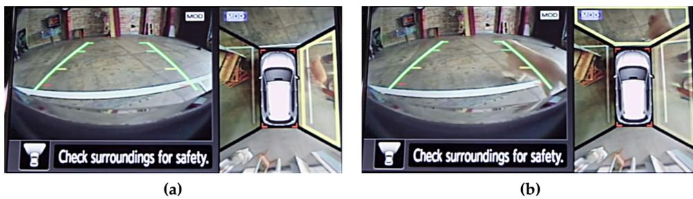
**Figure 5.15:** Example frames from Nissan’s Surround View Monitor. Note that the dog that appears on the right in (a) looks vastly different when it moves to the front in (b) [13].
