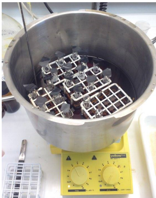
Figure 7.9: Setup for permeation tests with GO membranes and water as permeant.
