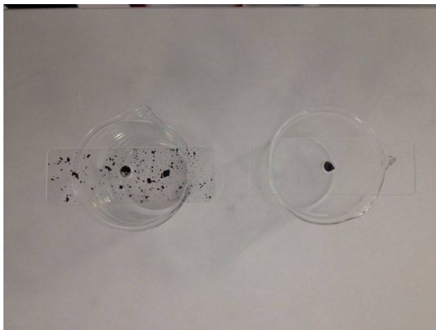
Figure 7.7: To the left is a crucible with 7mg GO which exploded during the heating to 220^{\circ}\text{C} , on the right is a crucible with 4mg GO which did not exploding when heated to 220^{\circ}\text{C}
