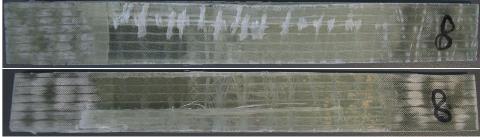
Figure C.44: Top picture is front view and bottom picture is back view of specimen 1-1-1_8 after testing has been performed. Fibre breaking has occurred close to the grips.
