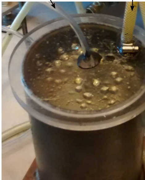
Figure 2.10: Outlet tube attached to the vacuum pump. Figure 2.11: Inlet tube attached to the pressure gauge.
