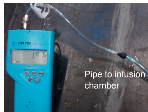
Figure 2.10: Outlet tube attached to the vacuum pump. Figure 2.11: Inlet tube attached to the pressure gauge.
