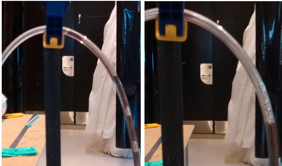
Figure 2.15: Vacuum pump at 100% and resin at high point. Figure 2.16: Vacuum pump at 60% and resin lower than figure 2.15
