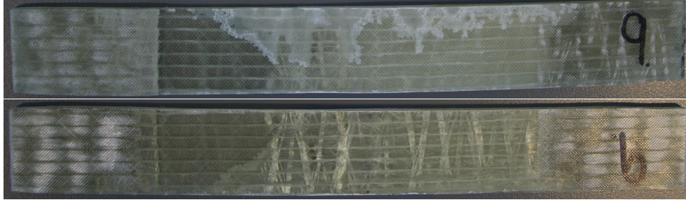
Figure C.51: Top picture is front view and bottom picture is back view of specimen 1-1-1_9 after testing has been performed. The white regions are remains from spray paint.
