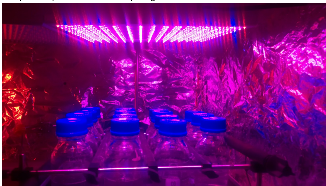
Picture 6 shows how the bottles were placed in the shaker during cultivation of A. platensis with different acetate concentration.
