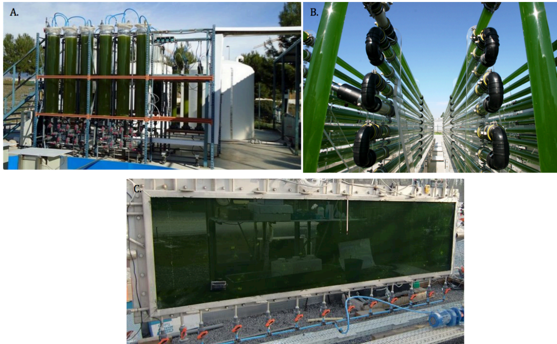
Picture 4 shows three types of closed photobioreactor system (A) Column photobioreactor (Yeomans, 2013). (B) Horizontal tubular photobioreactor (Bennekom, 2014). (C) Flat plate photobioreactor (AGICAL, 2013).
