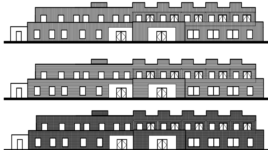
ill. 5.47: Different cladding materials
