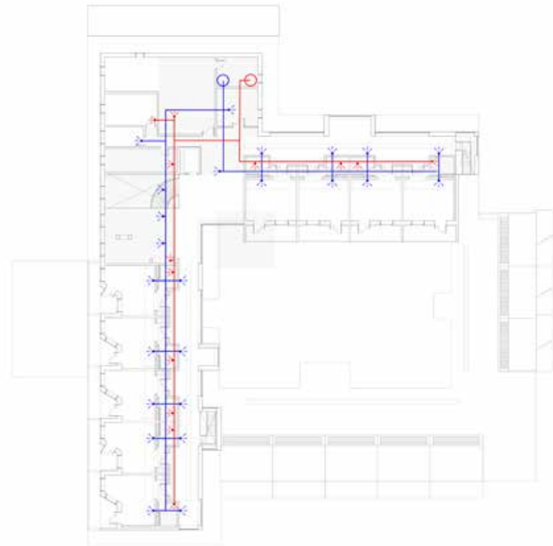
ill. 6.5: Ventilation pipes, first floor
