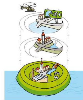
Figure 1.5: Multilevel safety. Level 1: prevention; level 2: sustainable spatial planning and -organization; and level 3: emergency management. Source: Oranjewoud & HKV Lijn in Water, 2011.
