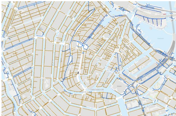
Figure 1.11: Sewer system city center Amsterdam. Brown: combined system; blue: rainwater system (own map).
