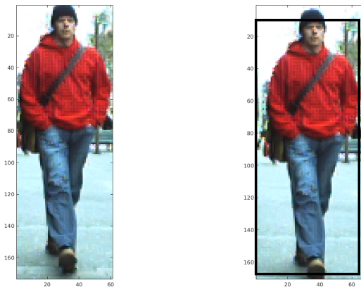
Figure 6.6: Confidence approximation for network result. Left: Network output. Right: Scaled bounding box. The black bounding box denotes the detectors approximation. The initial confidence is 68.19 and the final confidence is 66.9.
