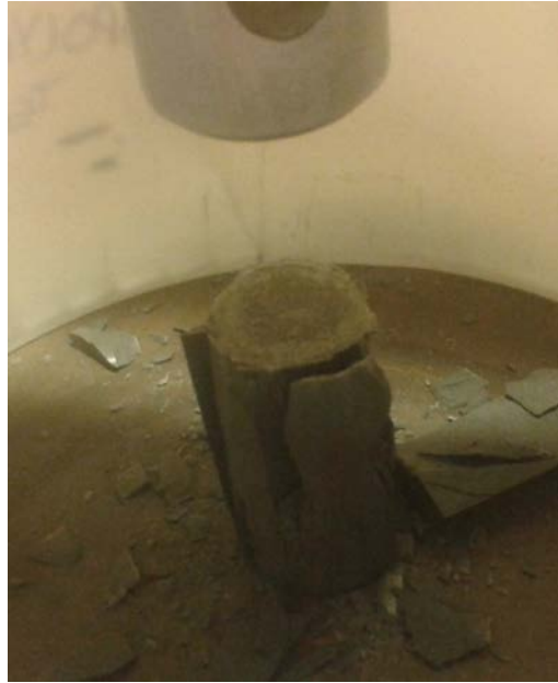
Picture 24-Failure pattern of mix design for GPC with NaOH 30% (cured at 7 days@90oC)
