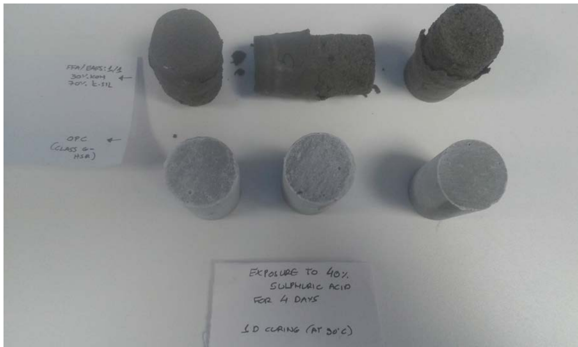
Picture 21-Samples after attack with 40% sulfuric acid
