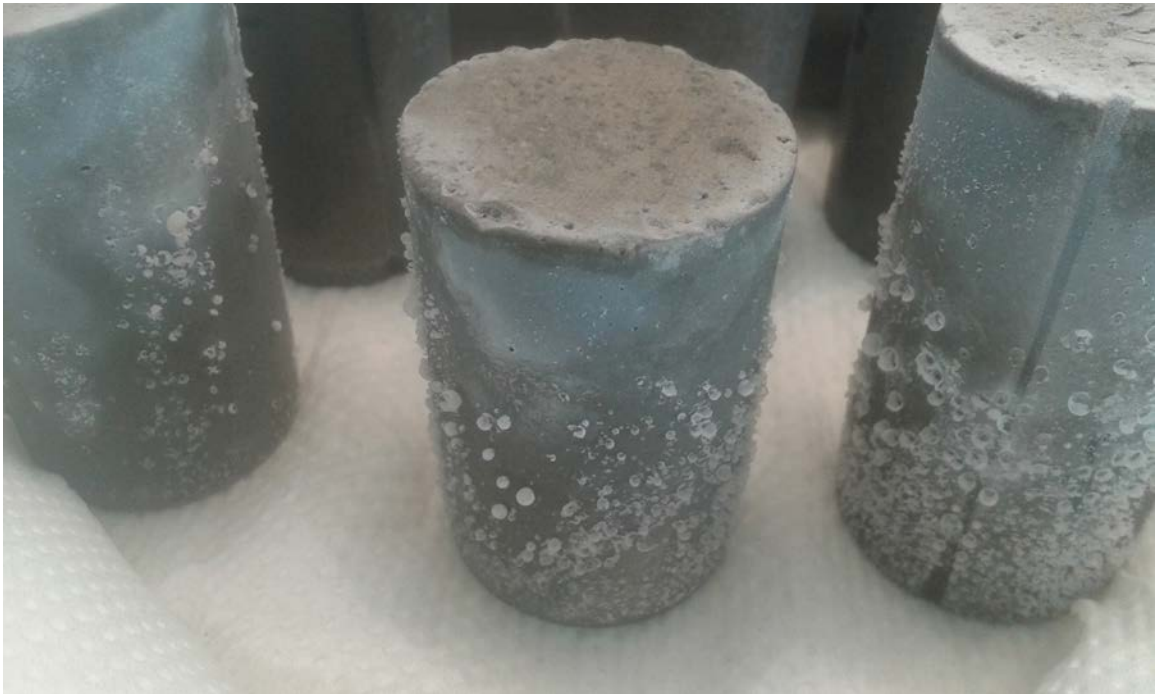
Picture 18-Surface deterioration of OPC after sulfate attack ( \text{MgSO}_4 ).
