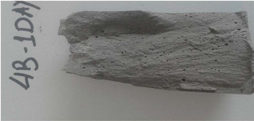
Picture 27- Pores are present despite the lowered amount of KOH (30% w/w)
