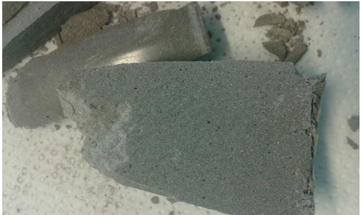
Picture 24-Structure of a crushed sample with FFA, KOH 6M and K-sil.
