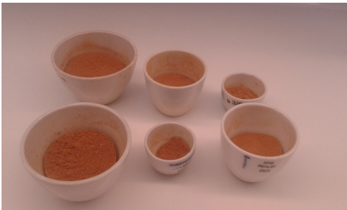
Picture 4-Samples of 2 different batches of FFA after exposure to 1050°C for LOI tests.
