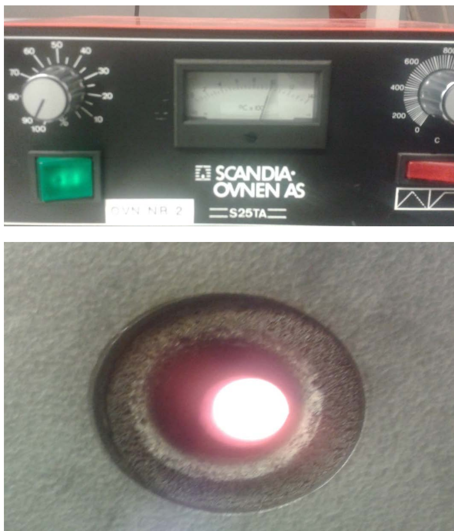
Picture 3-Furnace used for LOI measurements and high temperature curing
