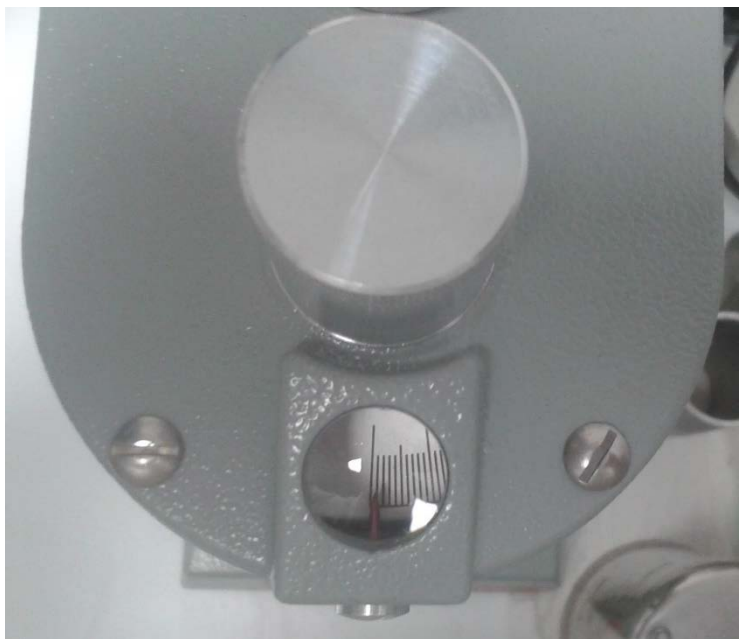
Picture 15-Fann 35A. Dial reading is almost zero. Maximum reading value is 300.
