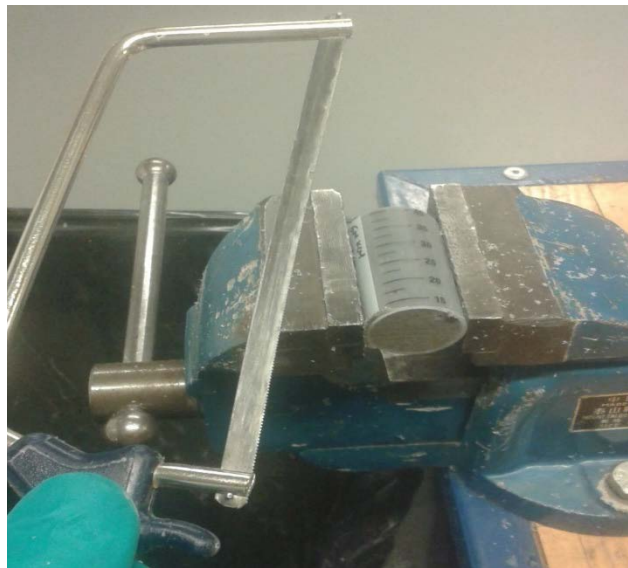
Picture 14-Demolding the samples with a saw (weak samples in danger of being damaged)
