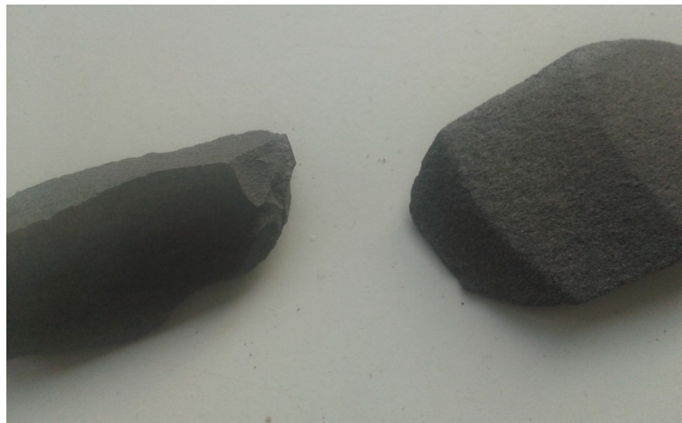
Picture 26-Effect of smaller particle size of EAFS (no pores visible)
