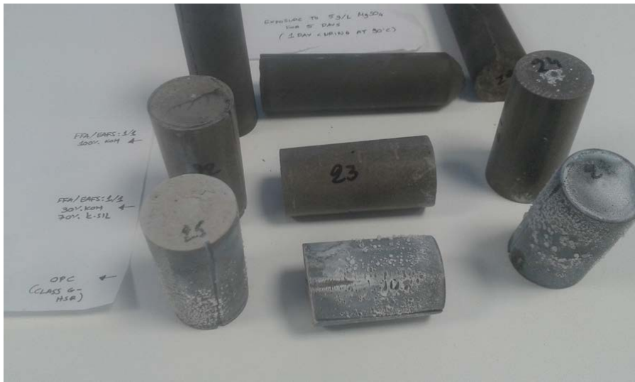
Picture 19-Different cement samples after exposure to MgSO_4
