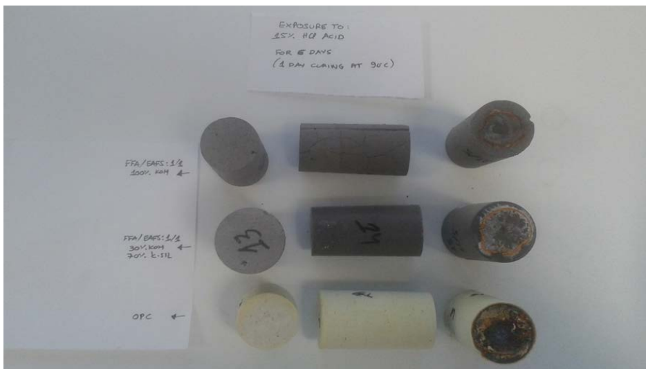
Picture 20-Samples after HCL acid attack
