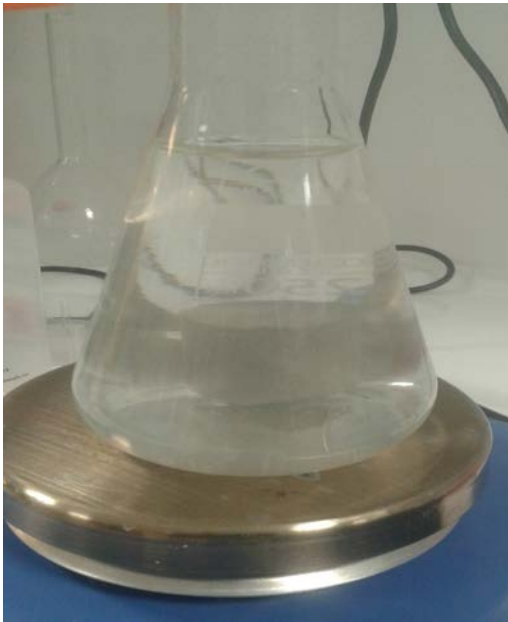
Picture 17-Boiling GPC sample for 1 hour to test long-term durability
