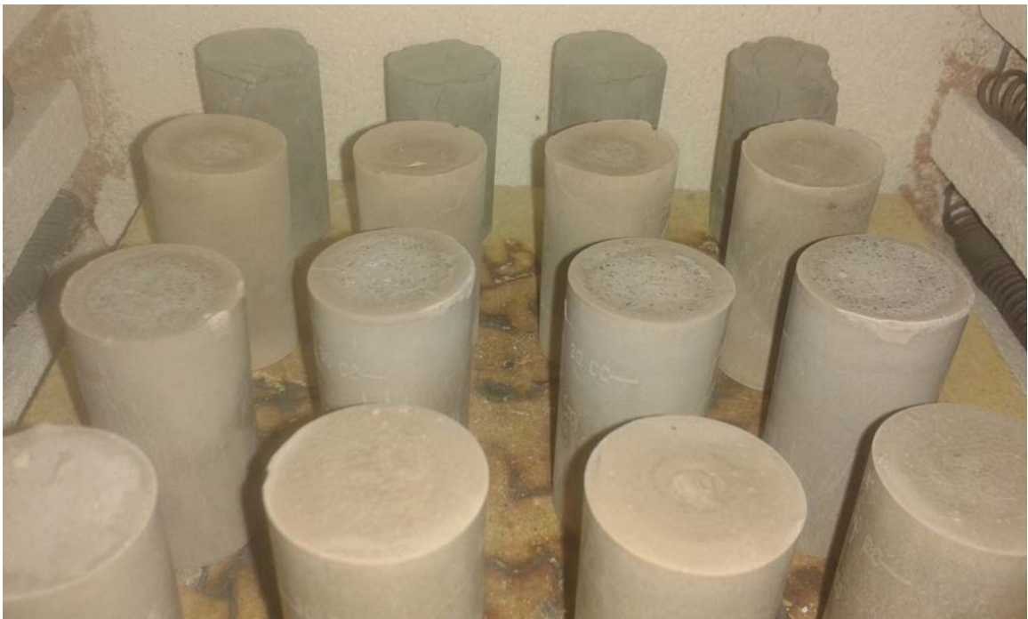
Picture 22-Samples after curing for 6 days at 400°C (1 day before were cured at 90°C).
