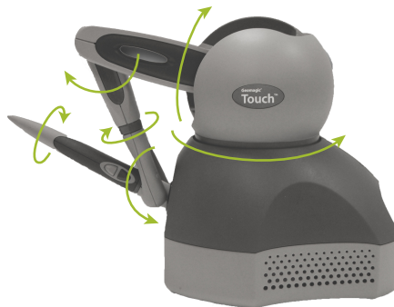
Figure 8.2: Representation of the 6DOF of the Geomagic Touch.
