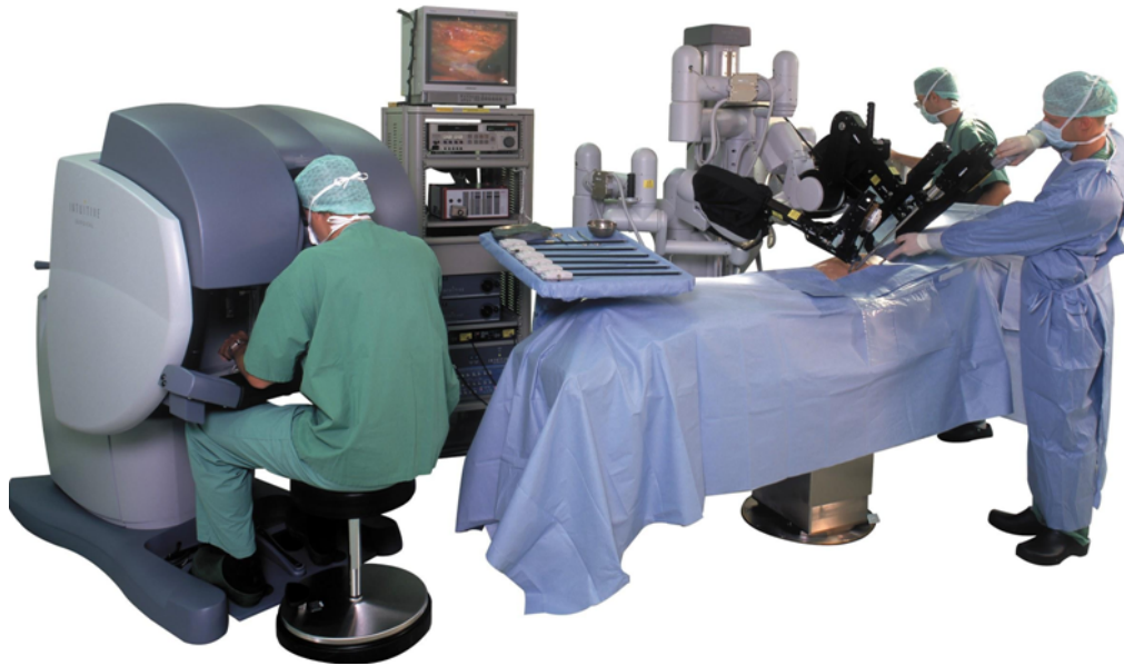
Figure 1.2: Da Vinci surgical System. On the left there is the surgeon master console where the surgeon can control the robot while looking to a 3 dimensional image. On the right, the robotic manipulator is following the trajectory given to operate a patient.
