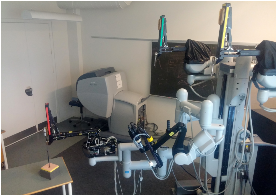
Figure 2.1: 1st generation of the da Vinci Surgical System at Aalborg University.
