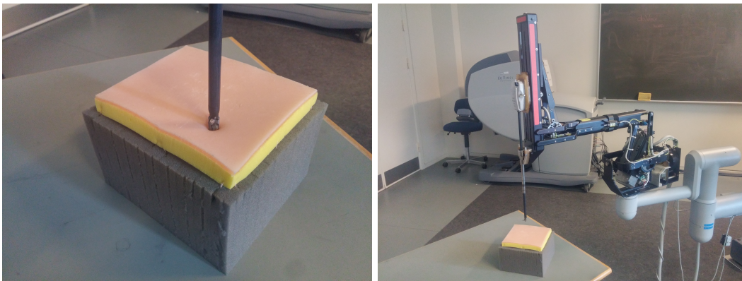
Figure 8.11: Tissue used to test the vertical movement of the da Vinci robot which is commanded by the haptic device.
