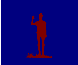
Figure A.8: Frame 700 segmented with a distance of 5 cm to the plane.
