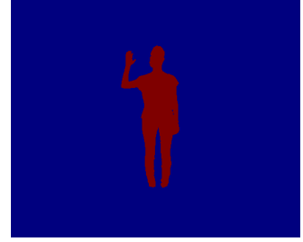
Figure 3.16: Frame 800 with removed points within 10 cm of the plane.
