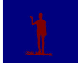
Figure A.3: Frame 200 segmented with a distance of 5 cm to the plane.
