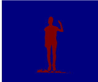
Figure A.14: Frame 300 segmented with a distance of 6 cm to the plane.
