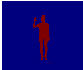
Figure A.26: Frame 700 segmented with a distance of 7 cm to the plane.
