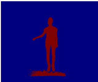
Figure A.16: Frame 580 segmented with a distance of 6 cm to the plane.
