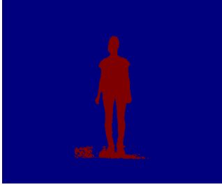
Figure 3.11: Frame 100 with removed points within 1 cm of the plane.
