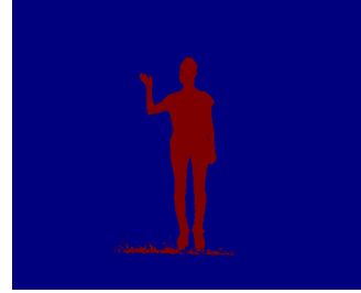
Figure A.12: Frame 200 segmented with a distance of 6 cm to the plane.
