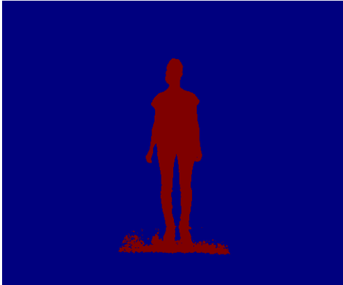
Figure 3.20: Frame 150 segmented with a distance of 5 cm to the plane.
