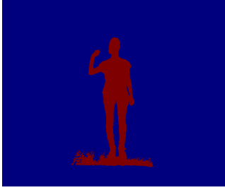
Figure A.1: Frame 70 segmented with a distance of 5 cm to the plane.
