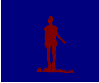
Figure A.4: Frame 285 segmented with a distance of 5 cm to the plane.
