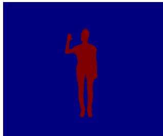
Figure A.53: Frame 700 segmented with a distance of 7 cm to the plane and noise removed.
