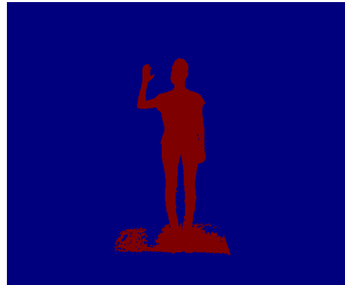
Figure 3.9: Segmented frame 800 based on the skeleton plus a margin of 20 cm in each direction.
