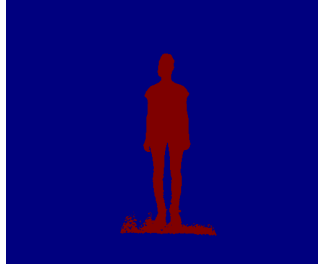
Figure A.2: Frame 150 segmented with a distance of 5 cm to the plane.
