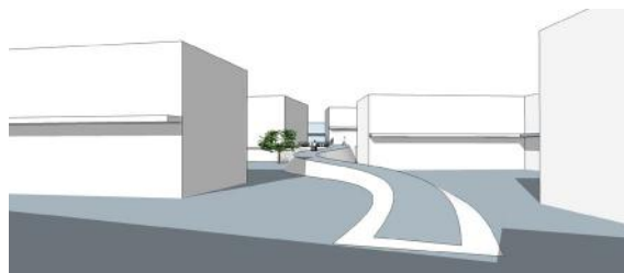
III.99. Curved ramp to take less place
