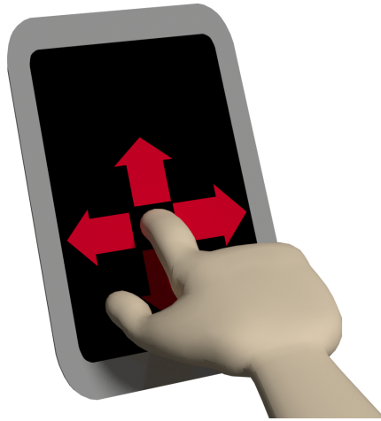
Figure 3.6: Click and drag interaction technique is used by swiping and moving a finger on the screen. Application calculates the movement with the finger and rotates the camera accordingly.
