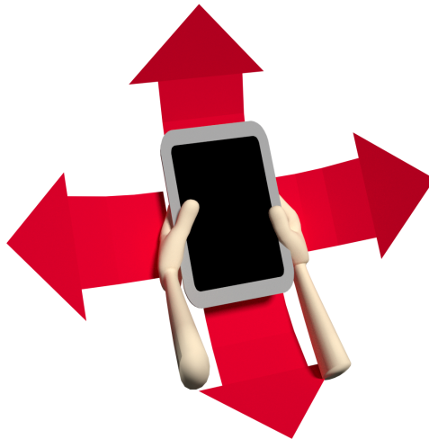
Figure 3.9: IMU-based rotation, and how the orientation and rotation is calculated with this technique. Tablet sensors calculate the relative movement done in the application and moves the camera in the application accordingly.
