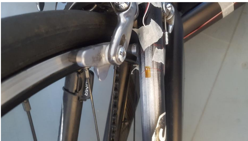
Figure 16 - Position of the quarter bridge SG at the front wheel.
