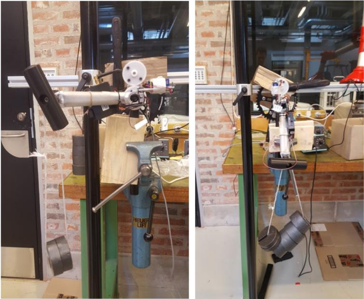
Figure 19 - Laboratory crank set calibration for the tangential (left) and radial (right) force.
