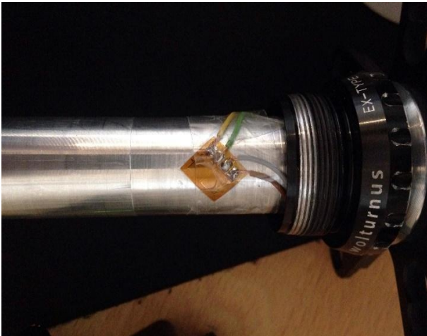
Figure 13 – Strain gauges position on the crankshaft.
