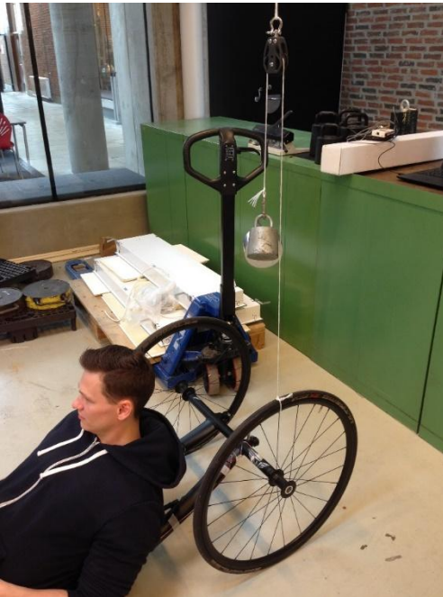
Figure 17 – Calibration setup for the rear wheel.
