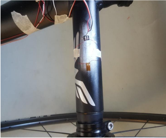
Figure 8 - Position of the quarter bridge SG at the rear wheel.
