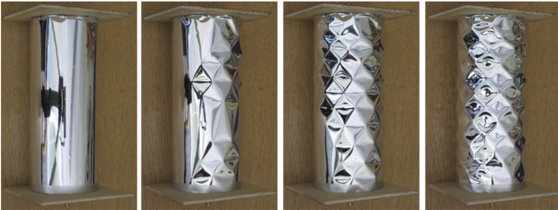
Figure 1.15: Buckling modes of a cylindrical shell [K. A. Seffen, 2010].
