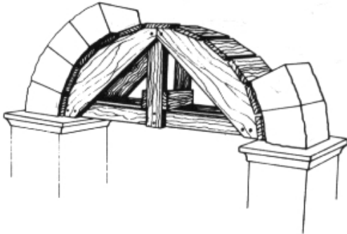
Figure 1.6: Circular arch with support during construction [Schillerinstitute, 2013].
