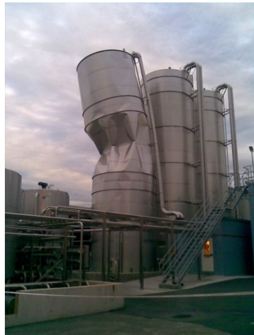
Figure 1.14: Buckling of shell structure [UCC, 2010].
