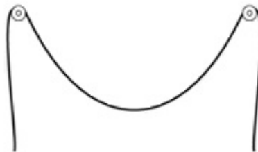
Figure 1.8: Chain hanging between two points creating the shape of a catenary [Schillerinstitute, 2003].
