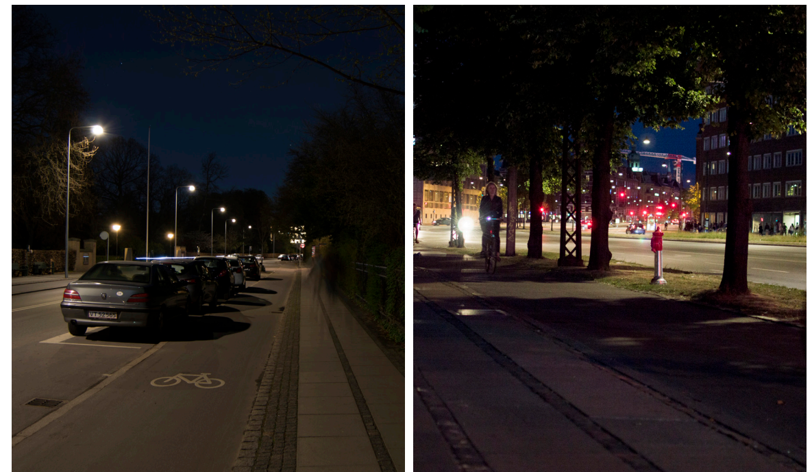
III. 36 & 37. On Bülowsvej (left), parked cars and an asymmetrical pole configuration create sharp shadows that cover more than half of the bike lane's width. Enghavevej, wet roads increase this effect by causing specular reflections of light sources. On Gyldenløvesgade (right) trees cast shadows that leave an entire stretch bike lane and sidewalk in the dark.
