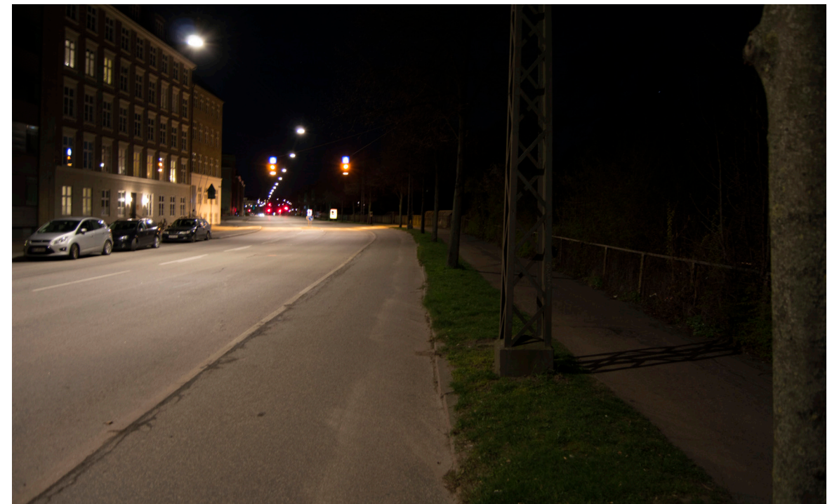
III. 29. On Øster Voldgade , the bike lane is relatively lit, but the light does not provide a sufficient amount of light on the adjacent footpath, making it difficult to rule out the presence of pedestrians. The low reflectivity of the dark surface on the footpath and a lack of viewing background contribute to the poor conditions.
