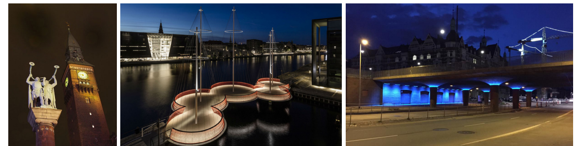
Ill. 49, 50, 51. Existing architectural qualities can be enhanced at night, by lighting them with neutral white light from a distance, like done at Rådhuspladsen (left). Other options include the integration of light in new constructions, to ensure from the beginning that they are designed with a day and night identity in mind from the beginning, as exemplified by the new Cirkelbroen (mid). A third option is to emphasize existing architectural qualities by giving them a new transformed identity by night, as exemplified by Jesper Kongshaug's lighting installation underneath Langebro, which uses colored light to create a unique night-time identity for a familiar piece of architecture.
