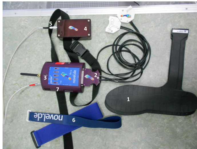
Figure 5.1: Pedar-X system: 1: insoles 2: Double insole cable 3: pedar-x box 4: battery 5: battery cable 6: velcro straps 7: SD card
