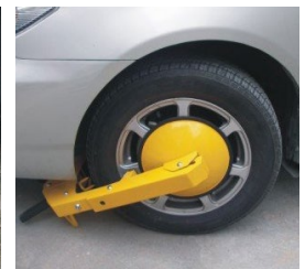
Ill. 72: Wheel locking shield.
