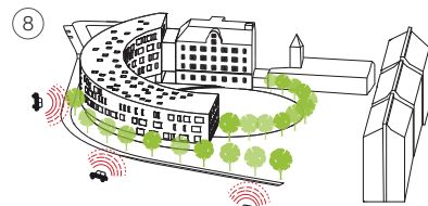
III. 10: Soft materials such as wooden terrace and trees around the building lessen the traffic noise.
