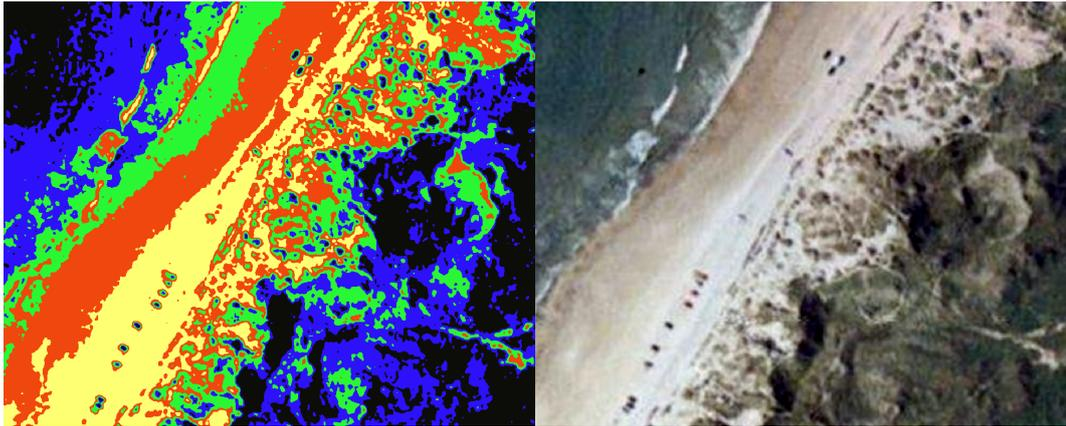
*Figure 7.13: Unsupervised classification using 5 (left) classes and the original image (right). 1995*
