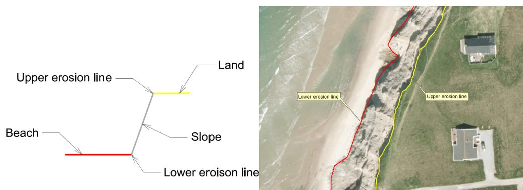
*Figure 5.2: The profile section of the erosion lines delimiting the land and beach (left) and the representation on the image*
