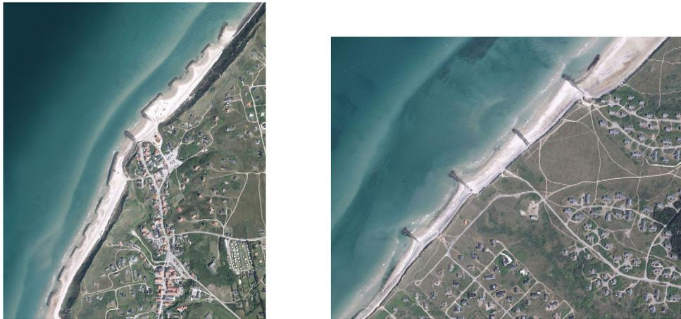
*Figure 2.7: Aerial imagery of Lønstrup town, the waterbreakers constructed starting from 1982 (left) and the groynes close to Skallerup Kilt (right)*
