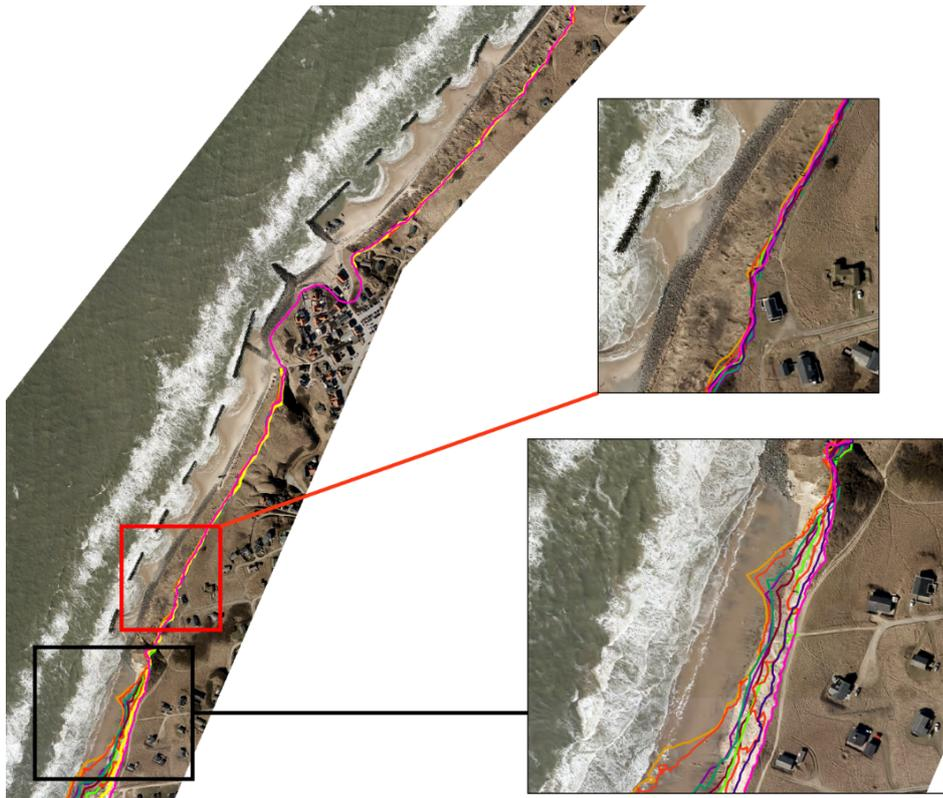
**Figure 9.9:** The erosion lines pattern along the protected area along with a detailed representation of the lines (red) and the erosion lines pattern along the unprotected area in the south of the waterbreakers (black)
