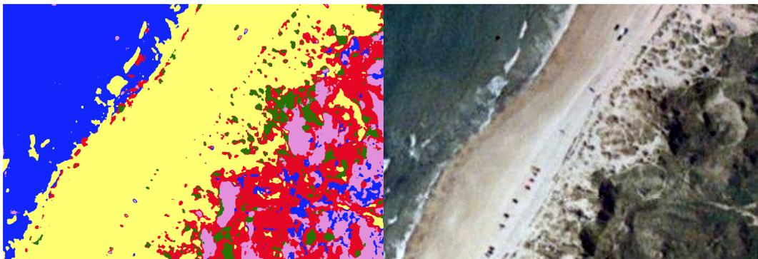
*Figure 7.9: Supervised classification using 5 classes (left) and the original image (right). 1995*
