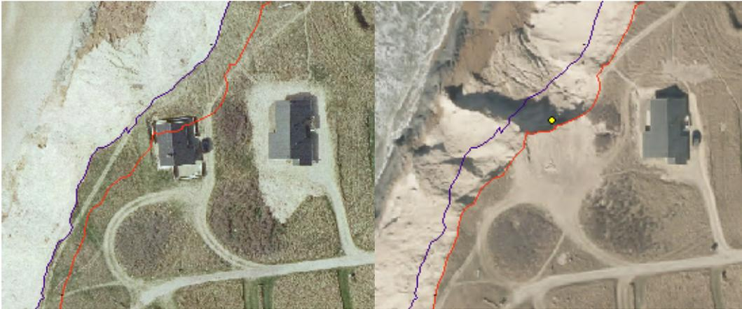
**Figure 9.15:** The house located between erosion lines 2012-2015 on orthophoto 2012 (left) and house loss registered on orthophoto from 2015 (right).
