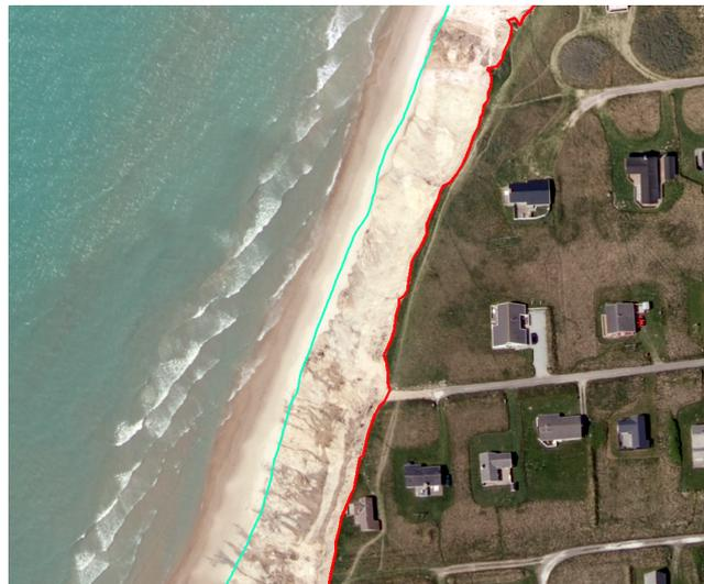
*Figure 9.2: The coastline extracted from the DEM (light blue) and the erosion line obtained from the image processing (red) 2006 data sets*
