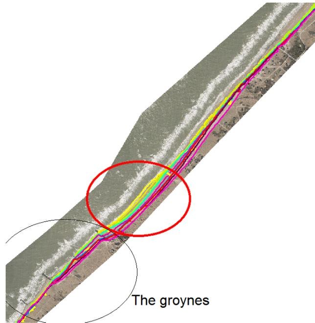
*Figure 9.12: Erosion lines pattern validate the lee side effect*
