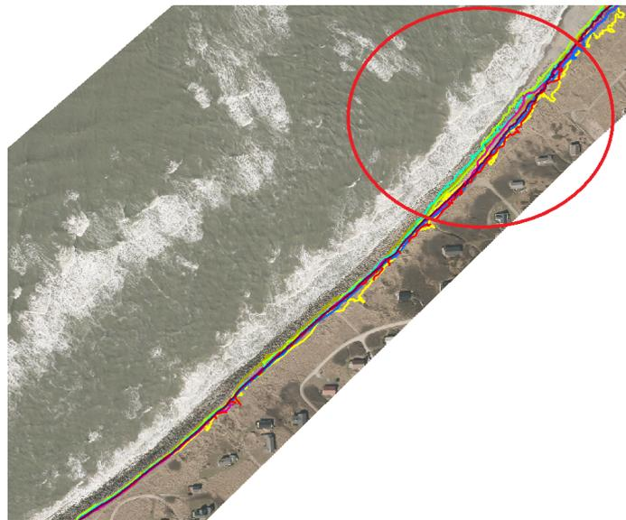
**Figure 9.10:** The erosion lines along the dam. As it can be seen in the upper part of the image, the erosion lines show a higher erosion, where the **dam protection ends**
