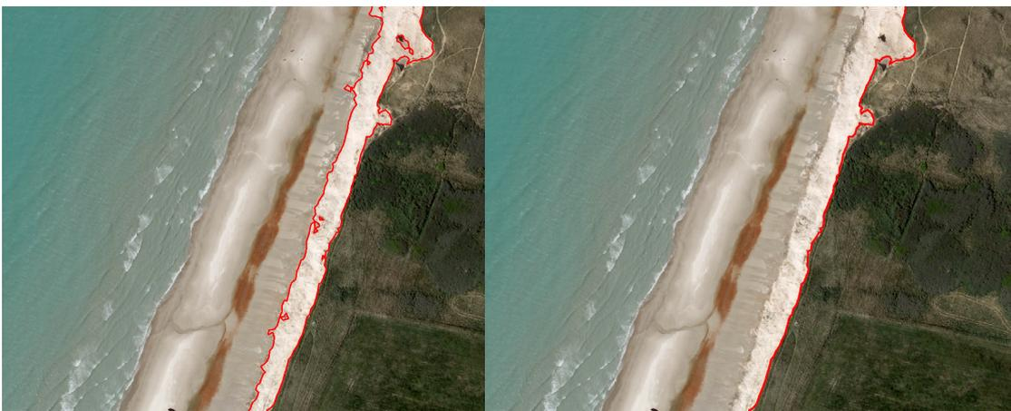
**Figure 8.4:** Transforming the polygons into lines (left) and the coast line mapped after the noise removal (right)
