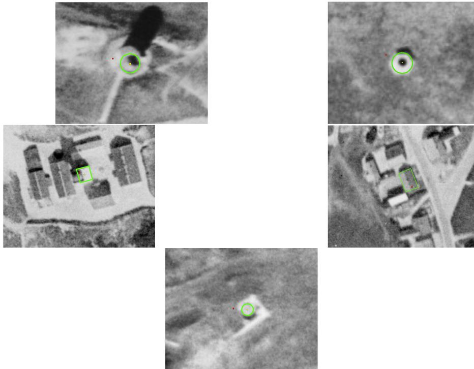
**Figure 4.11:** The translation difference between GPS points and objects on orthophoto from 1954.
