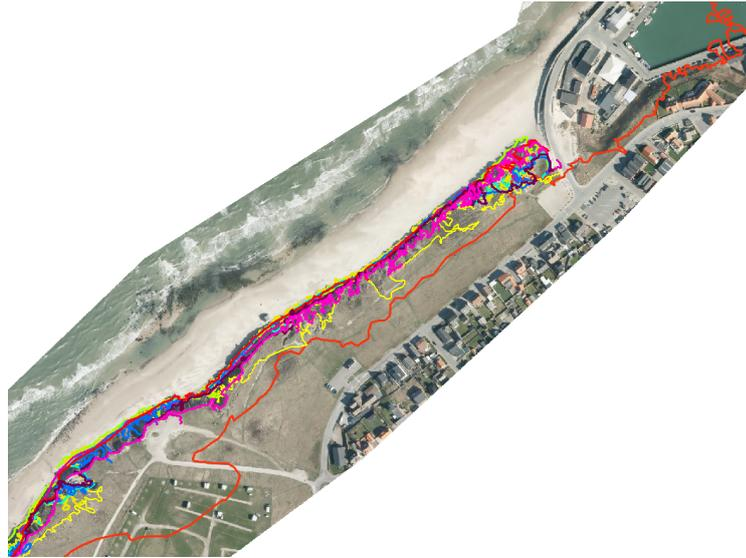
*Figure 9.13: The erosion lines showing the aggradation evolution. The red line is representing the erosion line from 1954*
