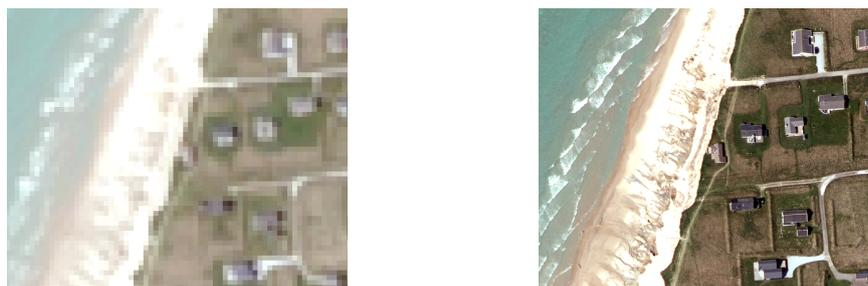
*Figure 4.2: The GSD quality from the image with 10000x10000 pixel (left) compared to the original orthophoto (right) with GSD quality 12.5cm*
