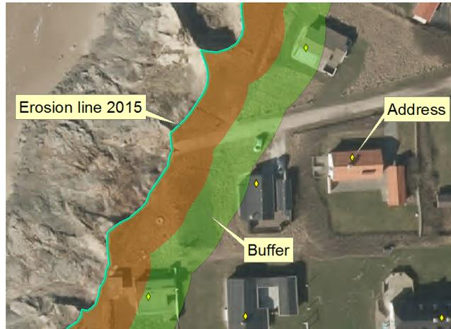
*Figure 9.18: The buffer line 10m and 20m in Lyngby area.*
