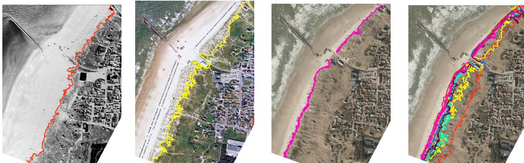
Figure 9.8: The erosion line according to the images from 1954, 1995, 2015, and the detailed evolution
