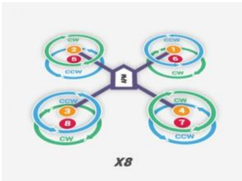
Picture 8. X8 UAV motors setup 12 .
