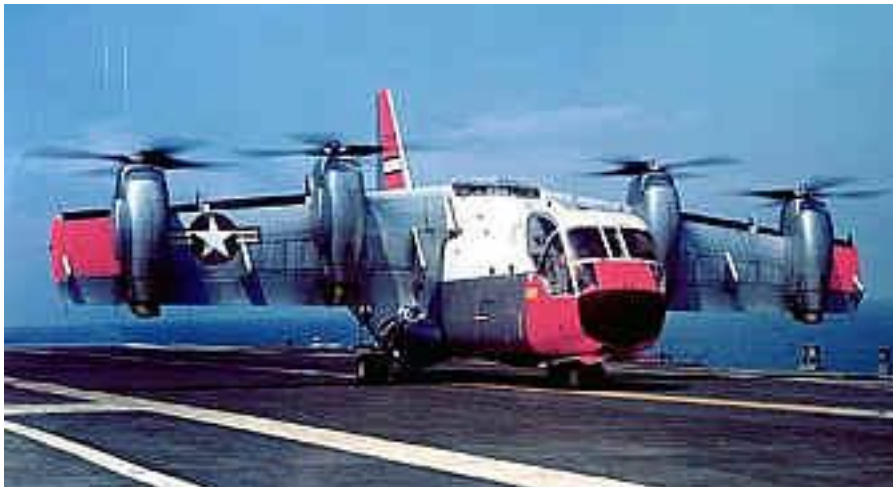
Picture 9. Tilt-wing VTOL 13 .
