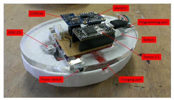
Figure 8 The hardware elements of Bean
