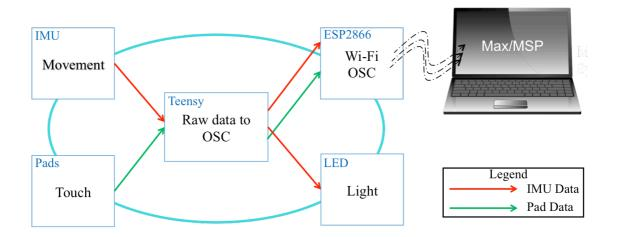
Figure 10 A visualization of the data flow in Bean
