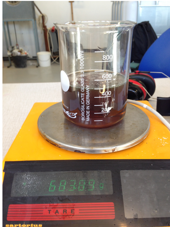
Figure B.1: 0.5 L oil on a weight scale for oil density determination.
