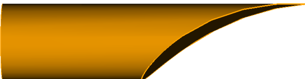
Figure 4.5: The inlet pipe to the hydrocyclone.
